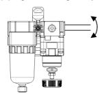
③ Non-flexible piping materials such as steel piping will be subject to excessive moment load and vibration from the piping side, so use a flexible tube for intermediate connections.
