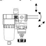
③ Piping materials without flexibility such as steel tube piping are prone to be effected by excess moment load and vibration from the piping side. Use flexible tubing in between to avoid such an effect.
