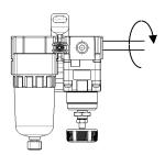
② Do not allow twisting or bending moment to be applied other than the weight of the equipment. Provide separate support for external piping, as damage may otherwise occur.
