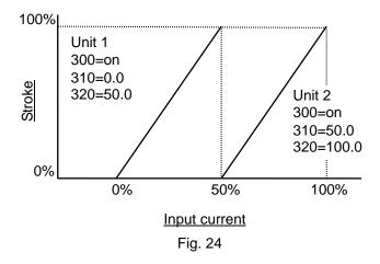
If the input current range is modified by setting the split range, an input value (S value) is shown with determination of the modified range as 100%. With the settings of (300) = ON, (310) = 0.0, and (320) = 50.0, it is reflected to each item as shown on Table 10. Suppose actuator full stroke is 30mm as an example.
