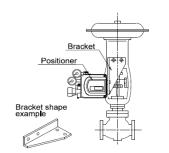
Attach using the screw hole at a side of the positioner and the screw hole at the front mount of diaphragm valve.
