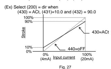
When this zero point / span setting is conducted, a position value (P value) is shown with determination of the set span as 0-100%. With the settings of (410) = vALu, (411) = 0.0, and (412) = 80.0, it is reflected to each item as shown on Table 12. Suppose actuator full stroke is 30mm as an example.
