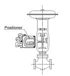
Directly attach using the screw hole at a side of the positioner and the screw hole at the yoke side of diaphragm.
