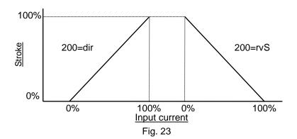
When the operation direction is modified, it is reflected on each item in accordance with Table 10. Suppose 30mm for actuator full stroke as an example.
