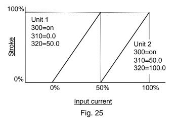
If the input current range is modified by setting the split range, an input value (S value) is shown with determination of the modified range as 100%. With the settings of (300) = ON, (310) = 0.0, and (320) = 50.0, it is reflected to each item as shown on Table 10.
