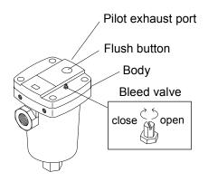
[Disassembly and cleaning of auto drain]
