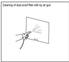
Fig. 8-3 Cleaning of the dust-proof filter
