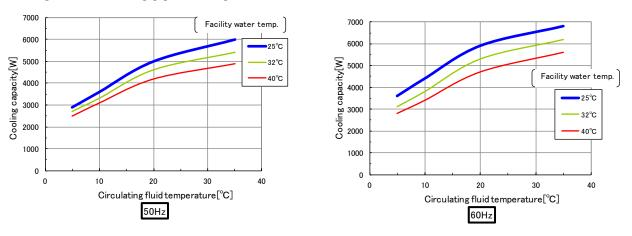
Fig 9-8 Cooling capacity (HRR050-W\*-20-\*)
