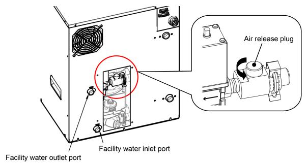
Fig. 8-4 Discharge of the facility water
