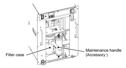
After discharging circulating fluid, insert the element into the resin filter case. Mount the resin filter case by hand tighten.
