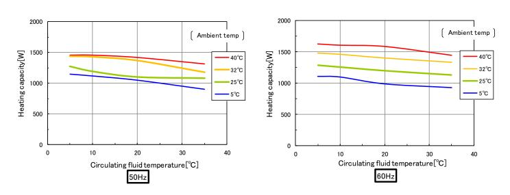
Fig 9-12 Heating capacity (HRR050-A/W\*-40-\*)
