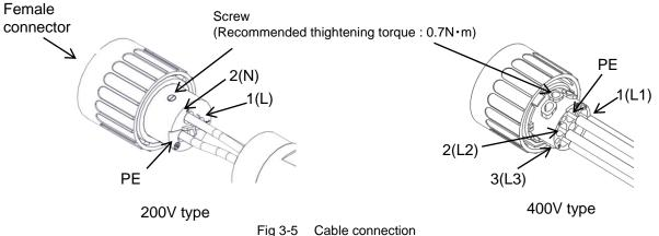
**5.** Assemble the power connector shell, gasket, ring and cable nut.
