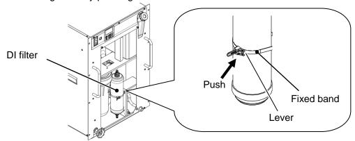
**3.** Pull out DI filter from opening of front side.
