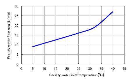
\*The amount of the facilitywater for the opution with rated circulating fluid, cooling capacity which is described in fig.9-8.
