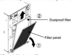
Fig. 8-2 Removal of the dust-proof filter
