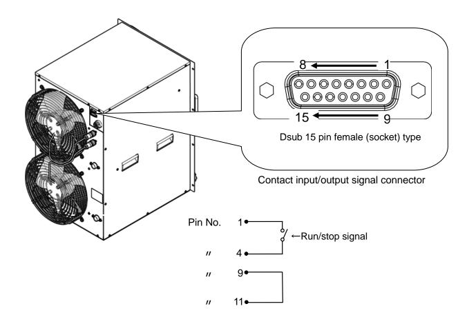
Fig 3-9 Wiring of run/stop signal input (Example)
