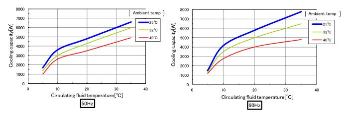
Fig 9-9 Cooling capacity (HRR050-A\*-40-\*)
