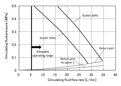
Fig 9-13 Pump capacity(HRR050-A/W\*-20-\*)
