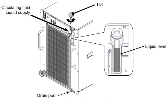
Fig. 3-15 Fill of circulating fluid
