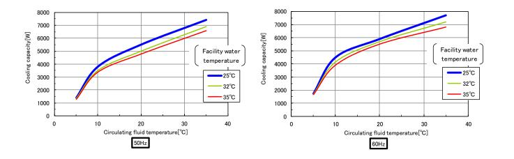
Fig 9-10 Cooling capacity (HRR050-W\*-40-\*)
