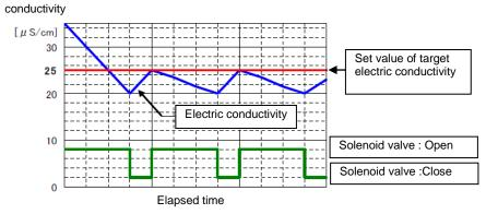
The solenoid valve for electric conductivity control can be made normally open/normally closed. (This function is available in operation.)
