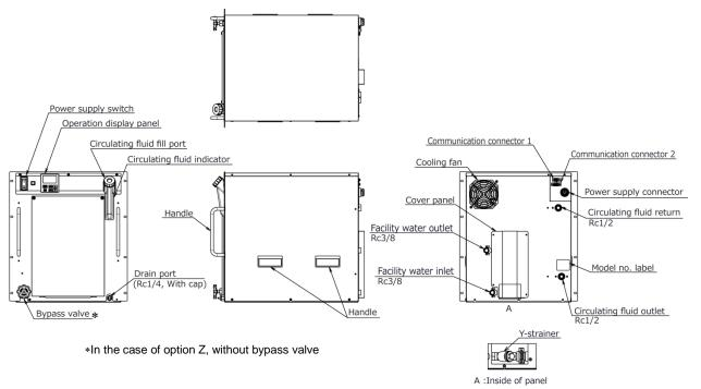
Fig 2-4 Names of the parts
