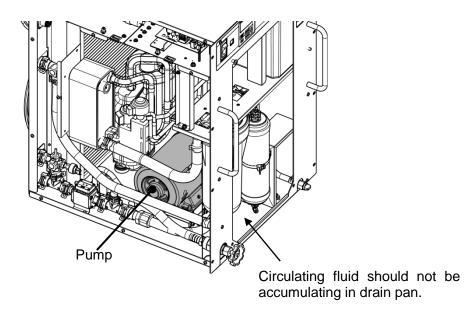
Fig. 8.2-4 leak check
