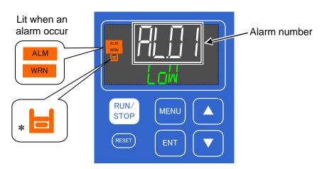
Fig. 7-1 Screen display of when an alarm occurs
