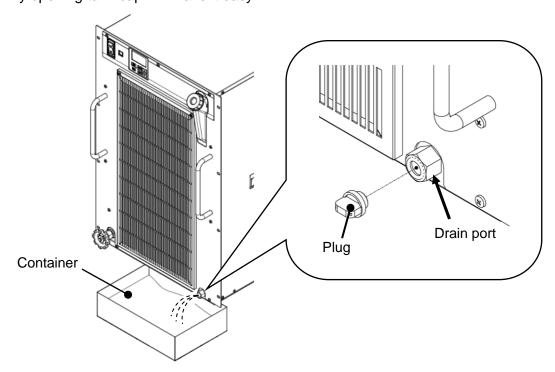
Fig. 8.3-1 Discharge of the circulating fluid
