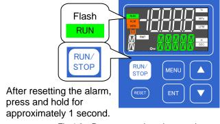
Fig 4-3 Restart operation when an alarm occurs
