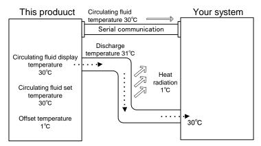
To switch the offset mode, press the [ENT] key. "OFF" flashes, press the [▲], [▼] key, select "OFF", "MD1", "MD2", "MD3" and confirm with [ENT] key.
