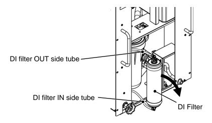
**4.** The connection fitting of the DI filter and the tube is connected by a fastener. O ring is used for the connection fitting. After removing the fastener, remove the connection fitting. Be careful not to apply force to the tube at this time. Also, please be careful not to damage the O ring.
