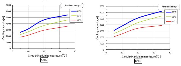
Fig 9-7 Cooling capacity (HRR050-A\*-20-\*)
