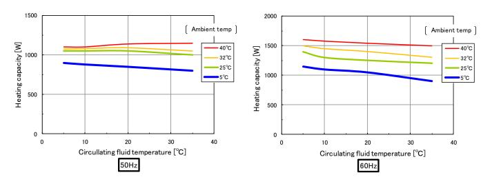
Fig 9-11 Heating capacity (HRR050-A/W\*-20-\*)
