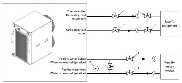
Fig. 3-14 Recommended piping circuit
