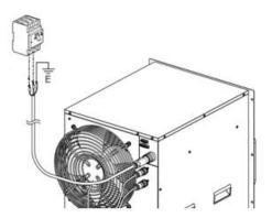
Fig 3-7 Power supply connector connection
