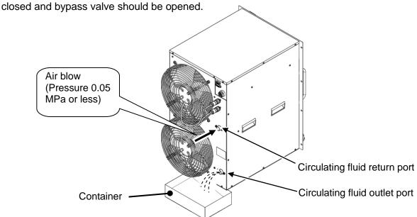
**4.** Particle filter is installed inside of this product. Discharge circulating fluid from inside of filter case. Remove filter panel holding screws by using cross slot screw driver and remove the filter panel.
