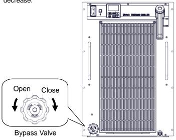
Fig 4-6 Adjustment of bypass valve
