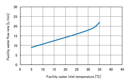
\*The amount of the facilitywater for the opution with rated circulating fluid, cooling capacity which is described in fig.9-10.
