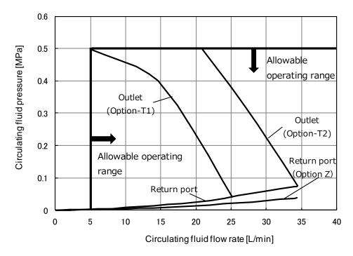
Fig 9-14 Pump capacity(HRR050-A/W\*-40-\*)
