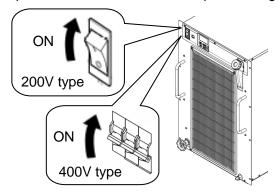
Fig. 4-1 Power switch location
