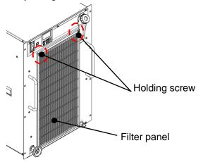
Fig. 8-1 Removal of the Filter panel
