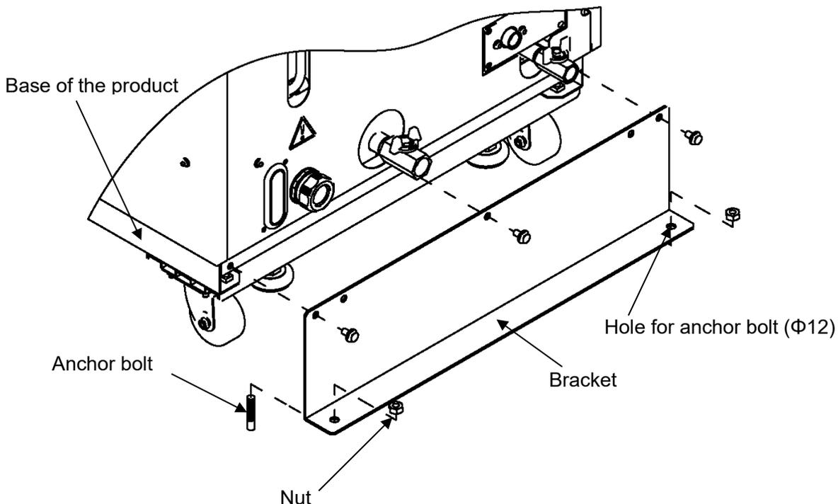
Fig. 3-4 Installation procedures
