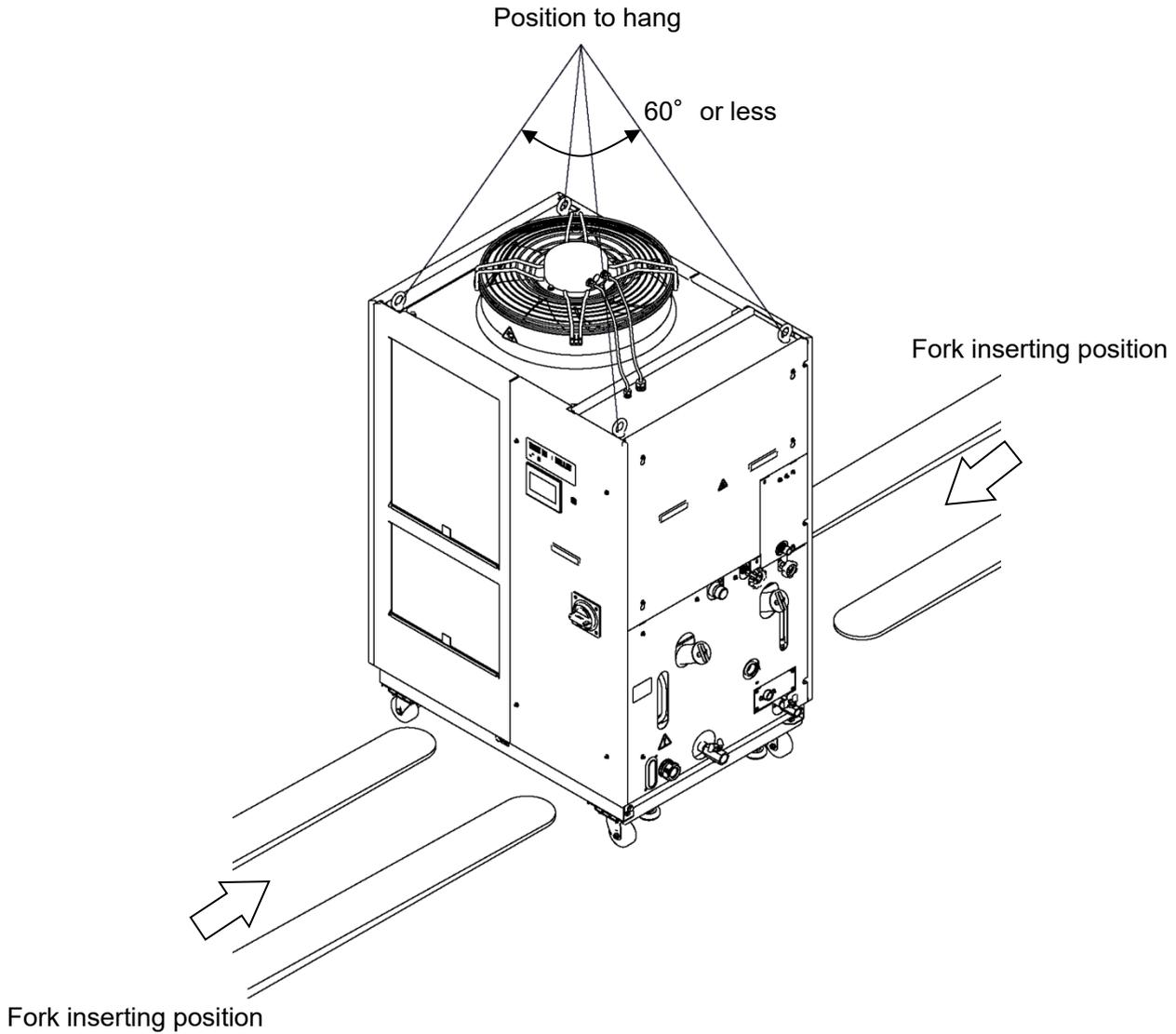
Fig. 3-1 Fork inserting and hanging position (This drawing shows “HRL200-A-20”.)
