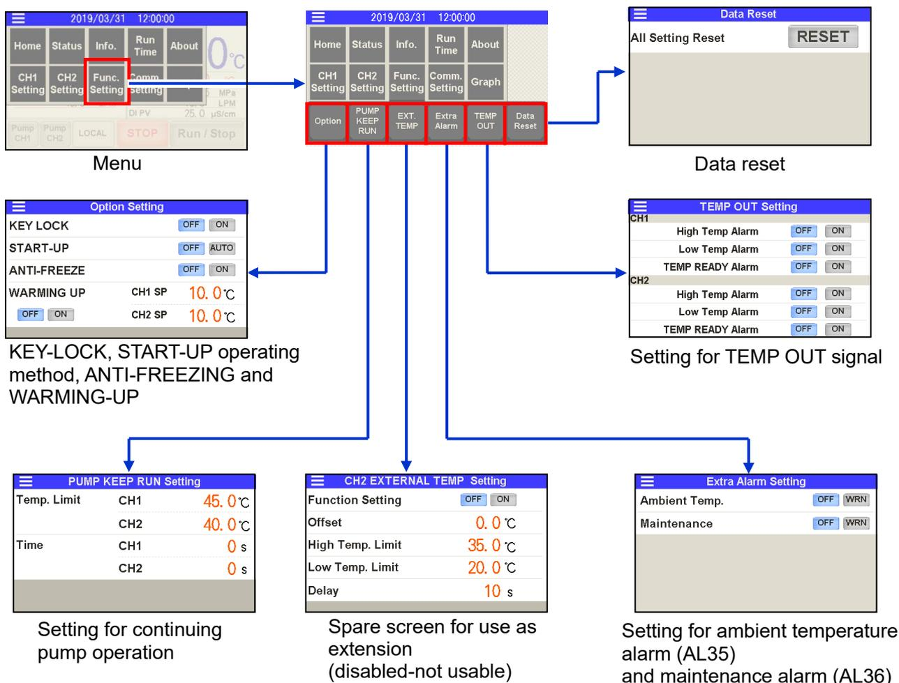
•KEY-LOCK, START-UP operating method, ANTI-FREEZING and WARMING-UP
