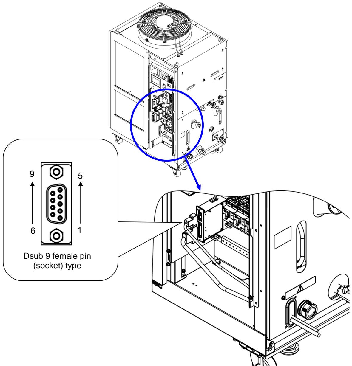
Fig. 3-12 RS-485 communication wiring
