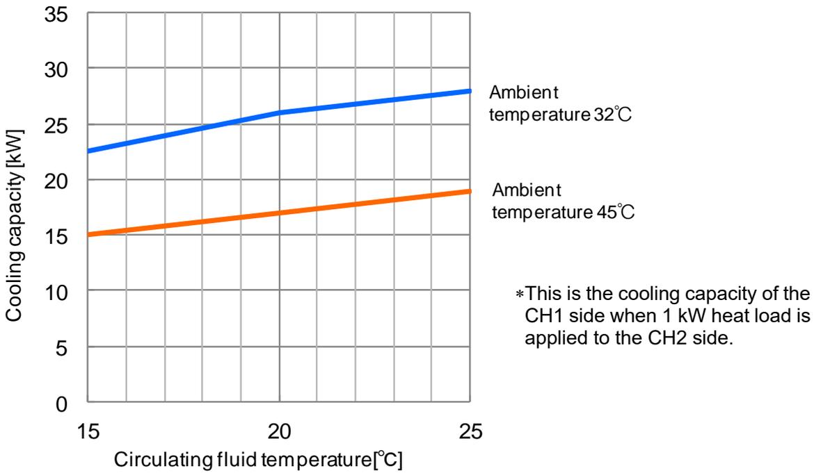
Fig. 8-7 Cooling Capacity (HRL300-A\*-20)
