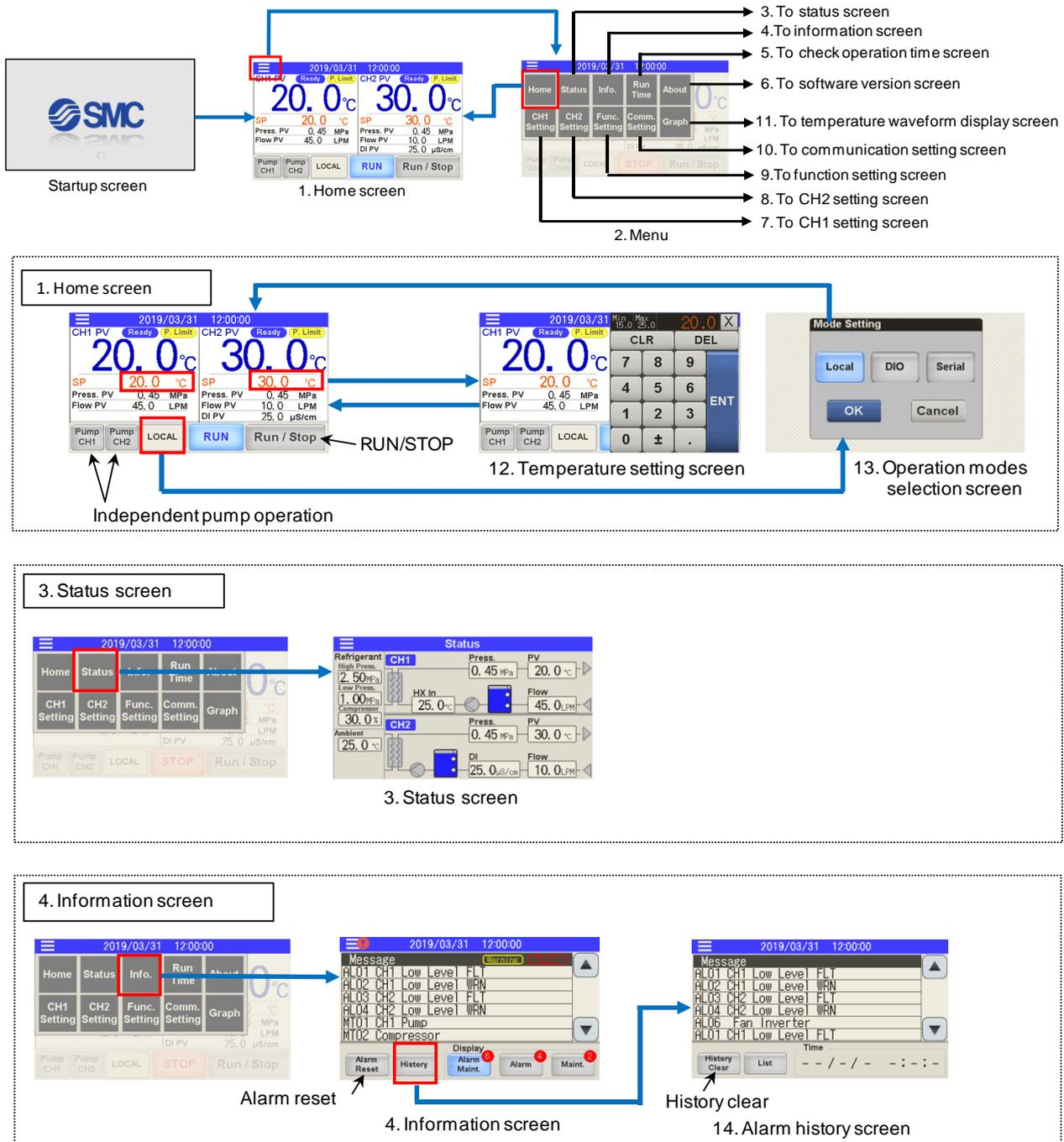
Fig.5-2 Flow chart of operation screen (1/3)
