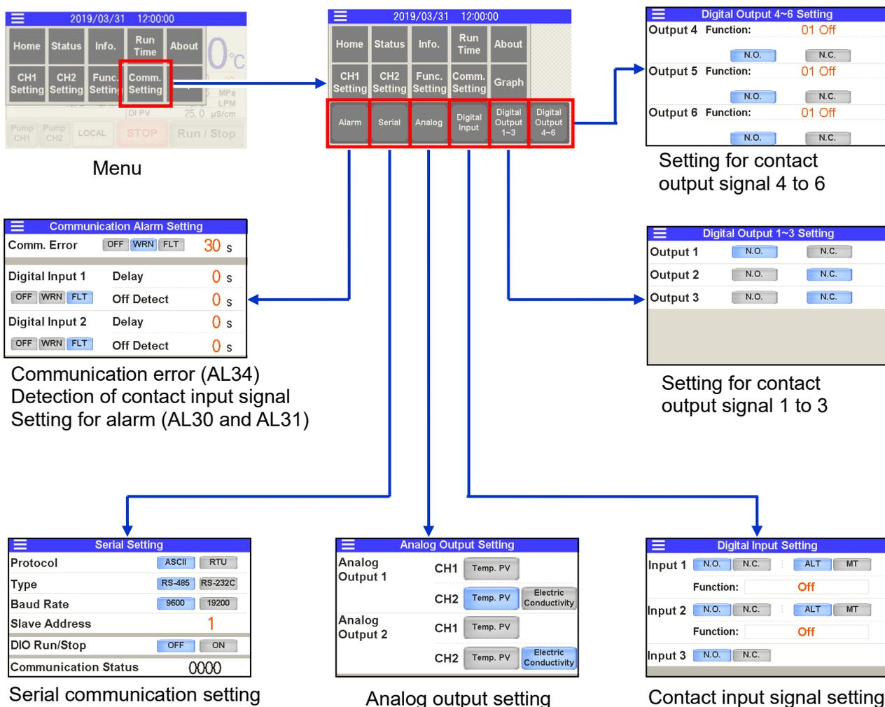
• Setting for communication error (AL34)/contact input signal detection (AL30 and AL31)
