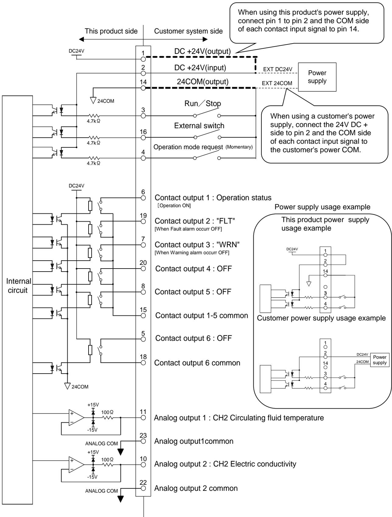
Fig. 3-10 Circuit diagram
