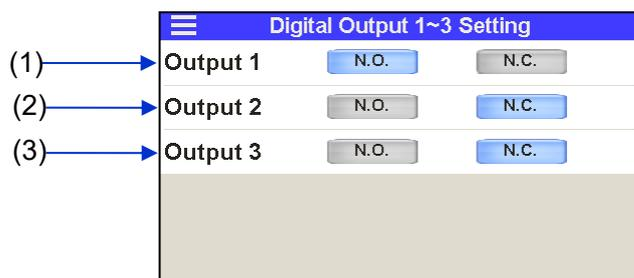
Setting of contact output signal 1 to 3
