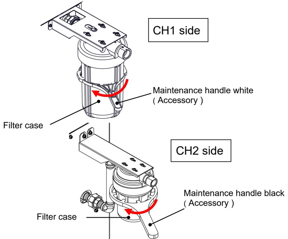
Fig. 7-3 Particle filter removal
