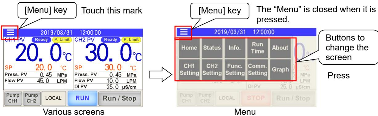
3. Press a button for example to carry out "Run/Stop," "Selection of function" or "Change the screen." Any button-shaped section on the screen can be pressed to operate it.
