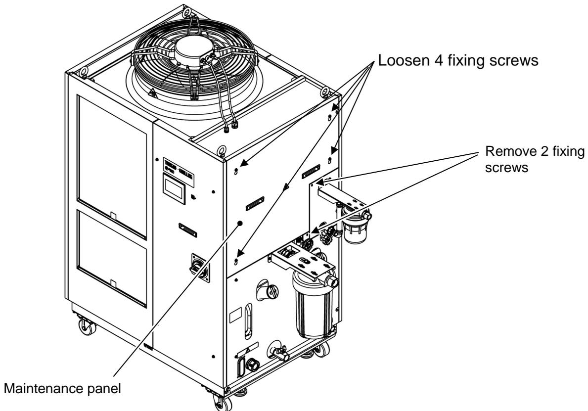
Fig. 7-5 Maintenance panel removal
