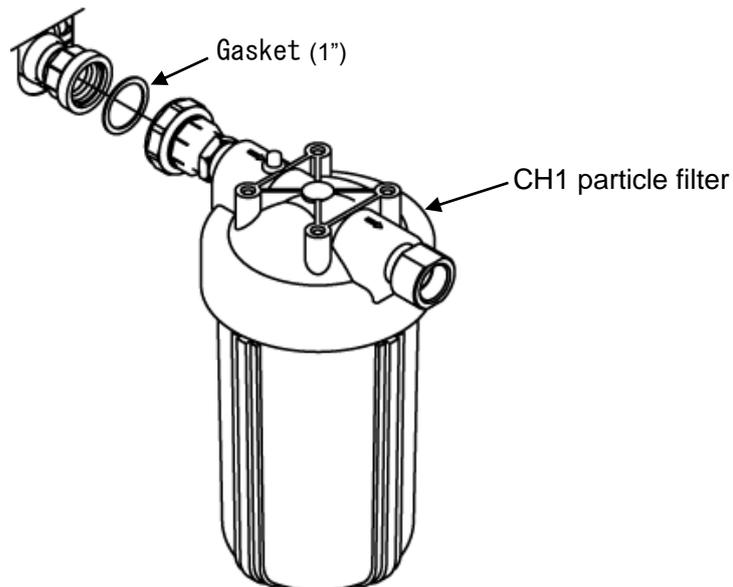
**3.** Attach the CH1 filter bracket.
