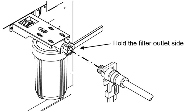
Fig. 3-17 Hold the filter outlet side
