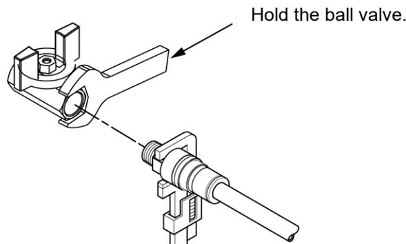
Fig. 3-18 Connection to the drain port
