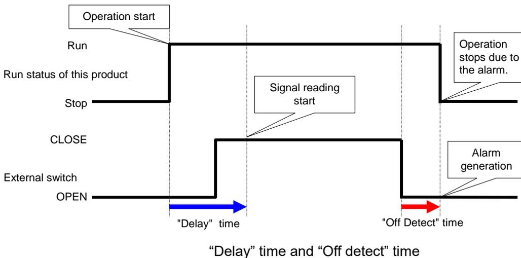
This function is set to “Disabled” by default. Refer to “Setting of contact input signal form” (P.5–55) for details. Contact input signal can be used to perform the “Run/Stop” of the product. Refer to “Setting of contact input signal form” (P.5–55) for the setting method.
