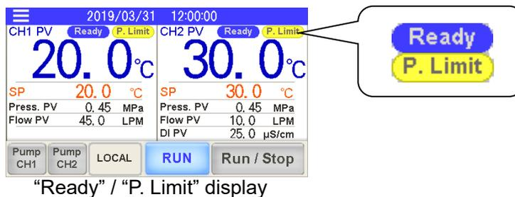
• Current circulating fluid temperature [PV]
