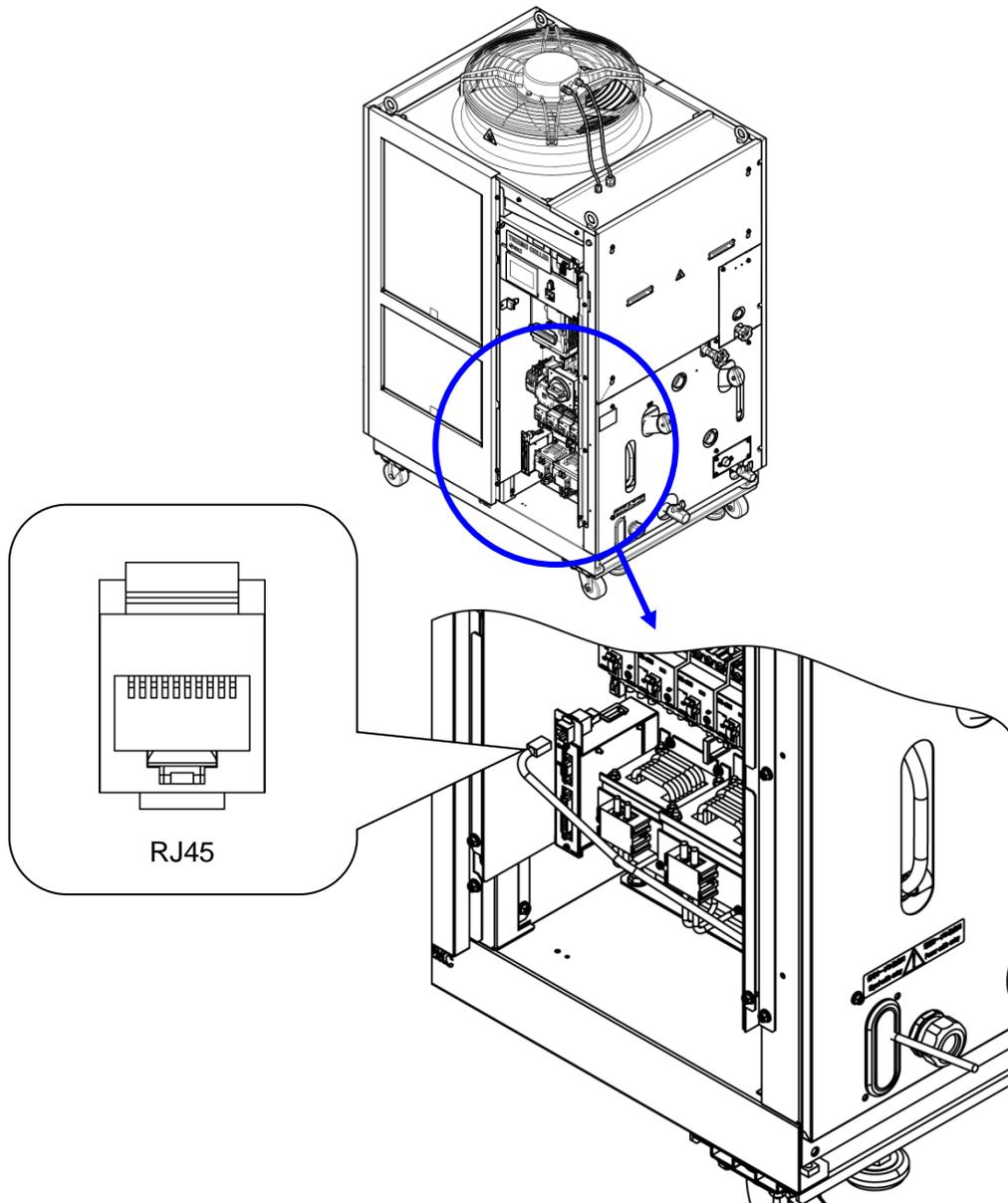
Fig. 3-15 Ethernet Modbus/TCP communication wiring
