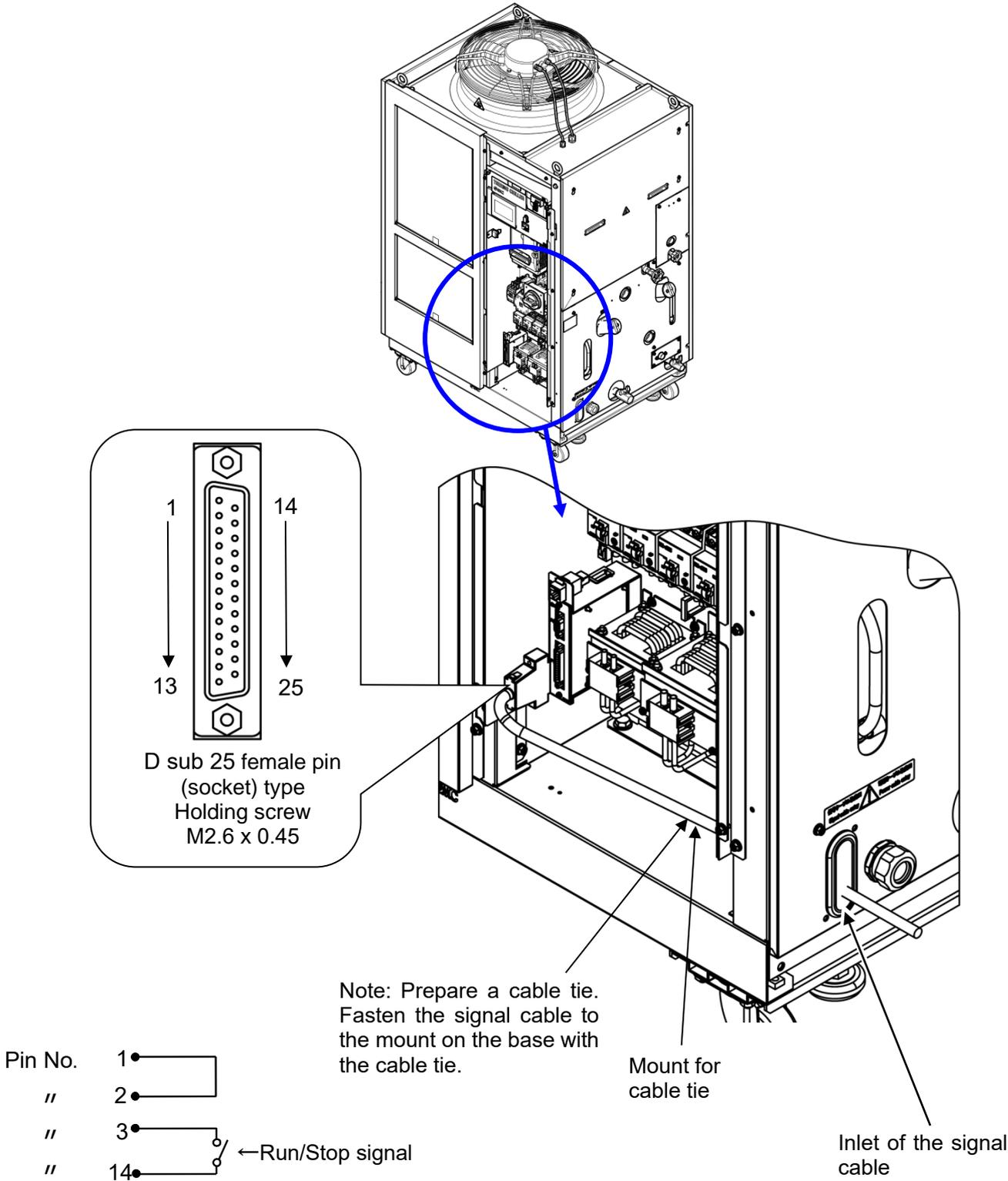
Fig. 3-12 Wiring of Run/Stop signal input and remote signal input (Example)
