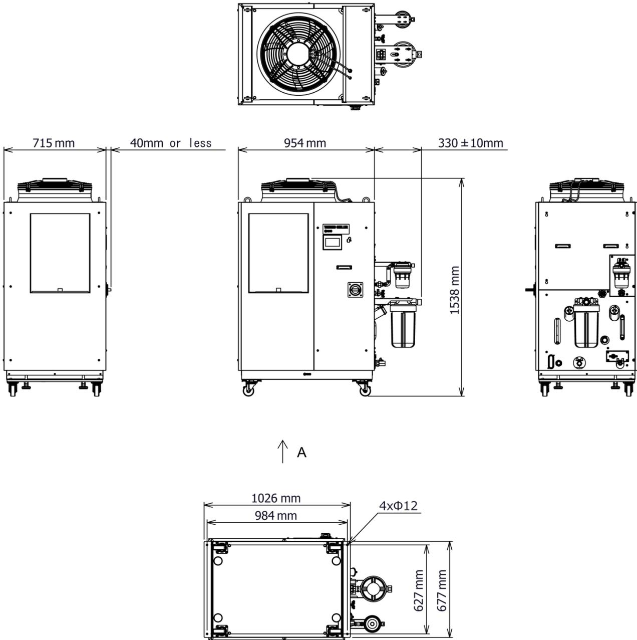
Dimensions for the positions of the anchor bolts (View A)
