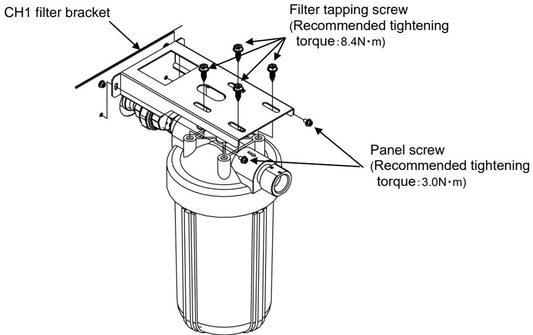
Fig. 3-18 CH1 side Installation of filter bracket.
