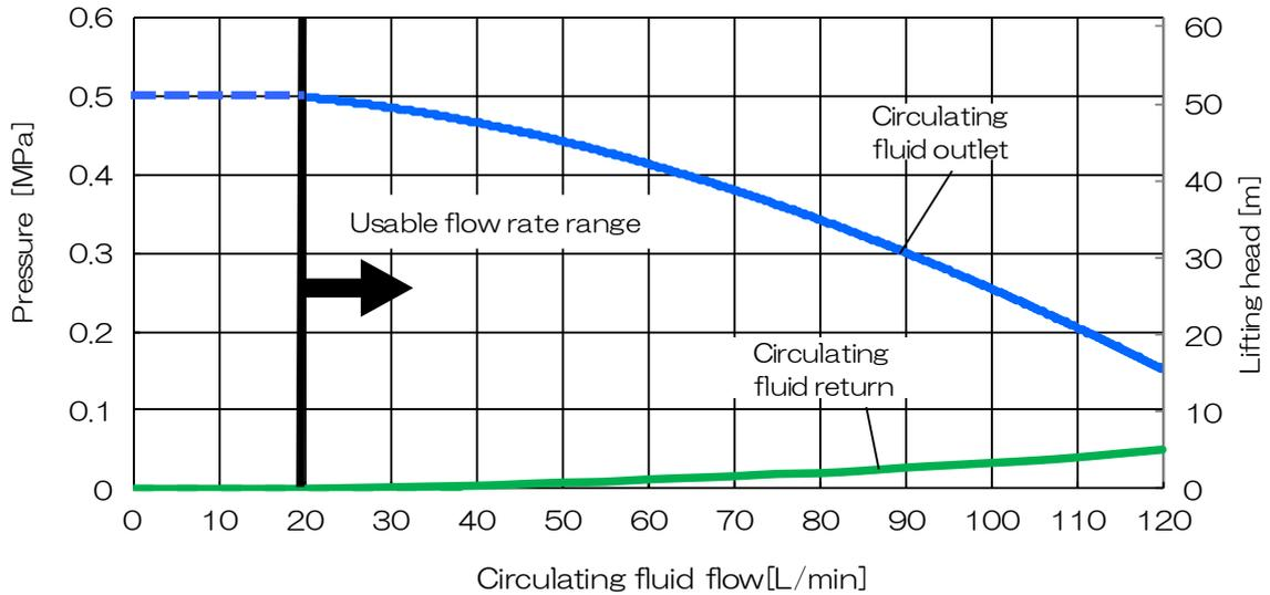
Fig. 8-9 Pump capacity(HRL100-A/W\*-20 CH1)
