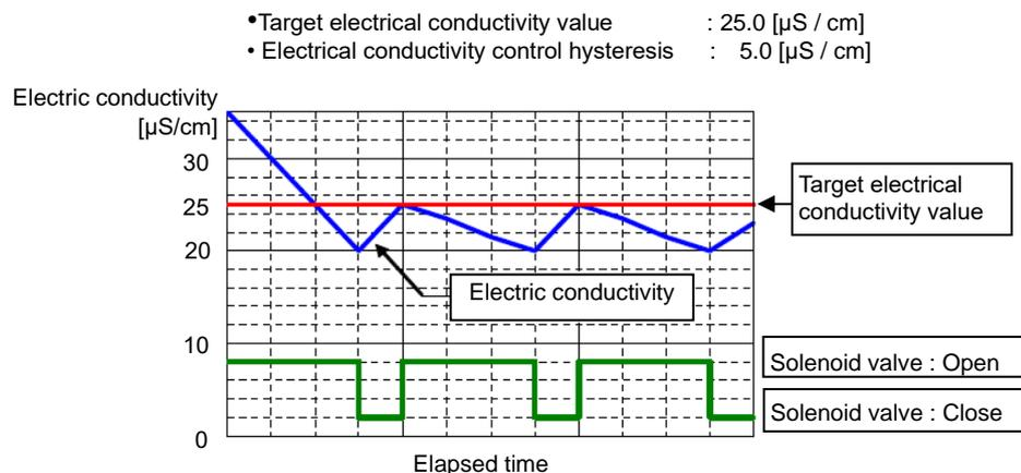
Fig.5-7 Example of electrical conductivity control
