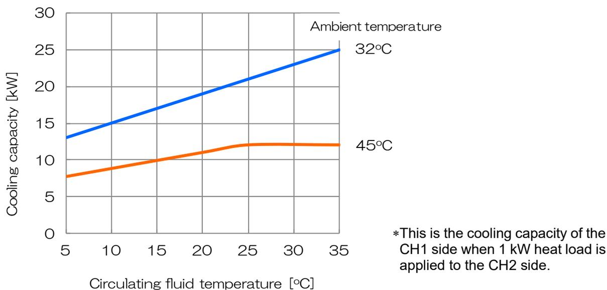
Fig. 8-8 Cooling Capacity (HRL200-A\*-20)
