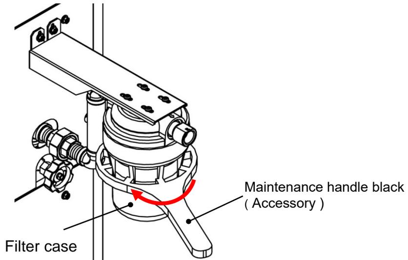
Fig. 3-23 CH2 particle filter case removal
