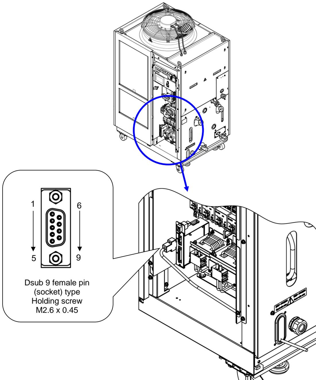
Fig. 3-13 RS-485 communication wiring
