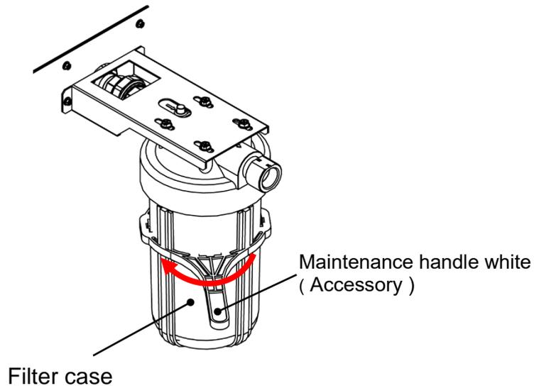
Fig. 3-22 CH1 particle filter case removal
