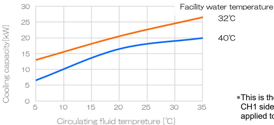
\*This is the cooling capacity of the CH1 side when 1 kW heat load is applied to the CH2 side.
