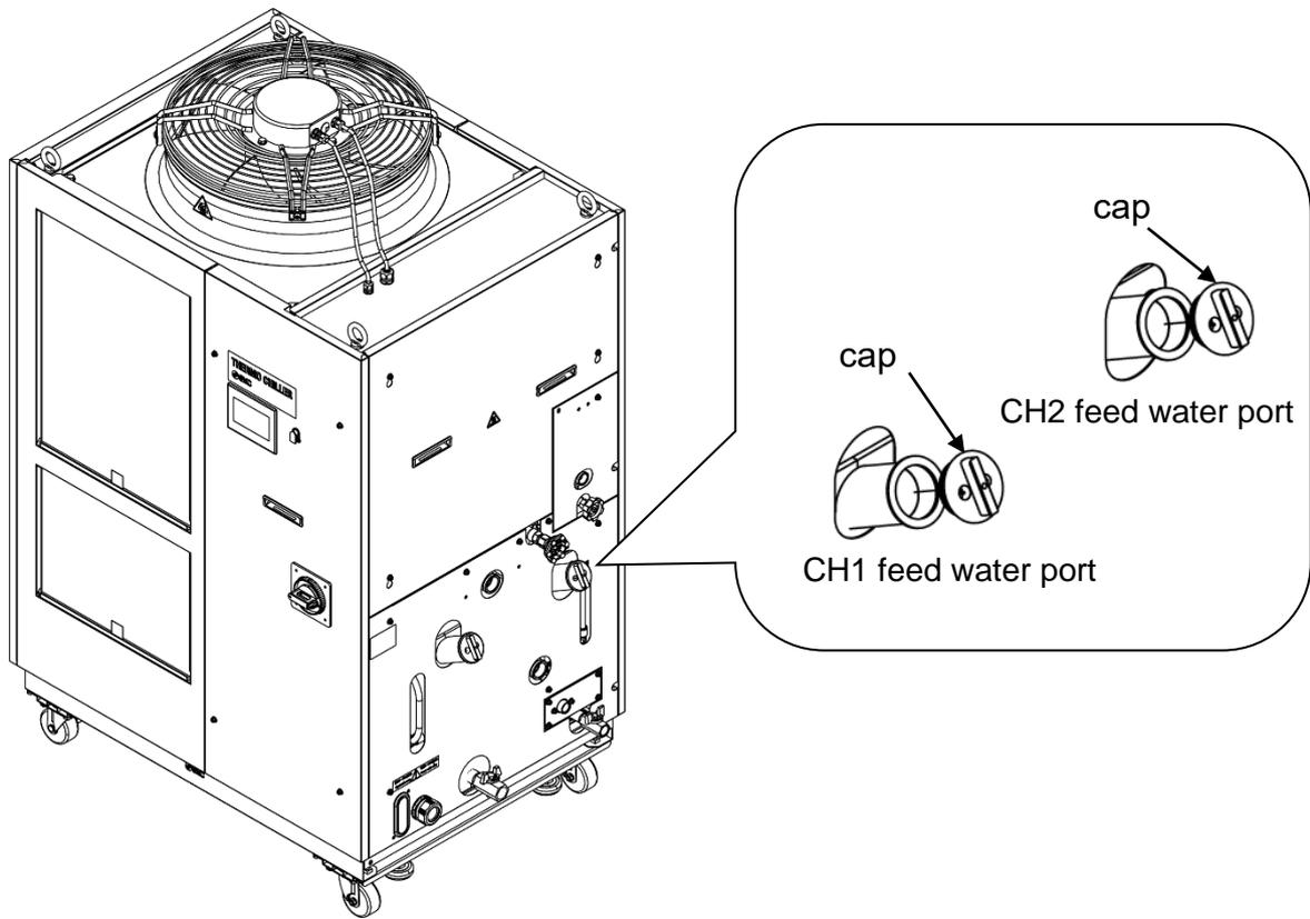
Fig. 3-28 Supplying the fluid to the supply fill port
