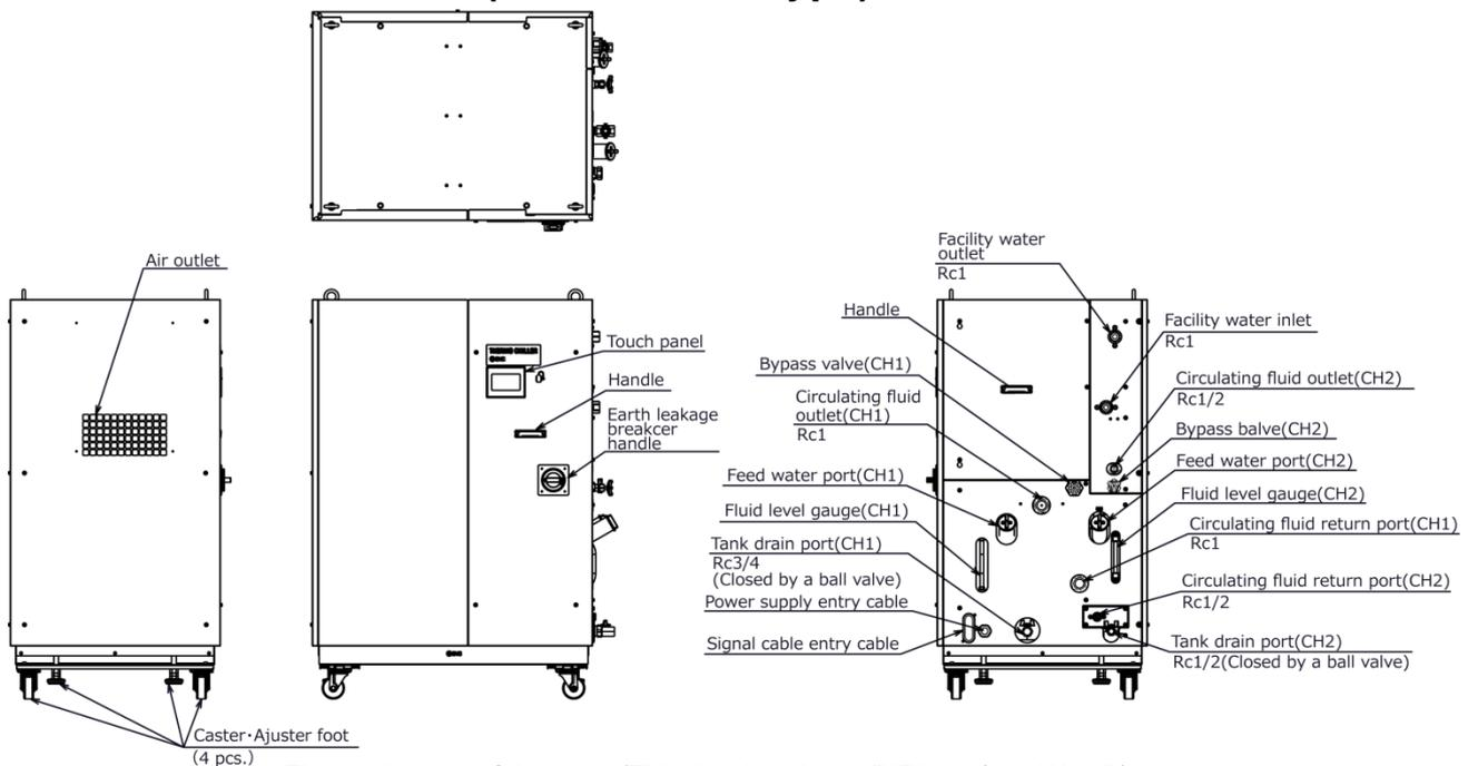
Fig. 2-2 Names of the parts (This drawing shows "HRL100/200-W-20".)
