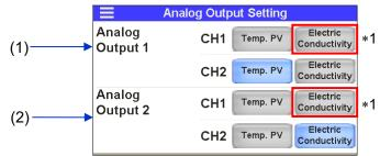
setting of analog output signal \*1 In the case of option D1 "CH1 with electrical conductivity control", it can be set.
