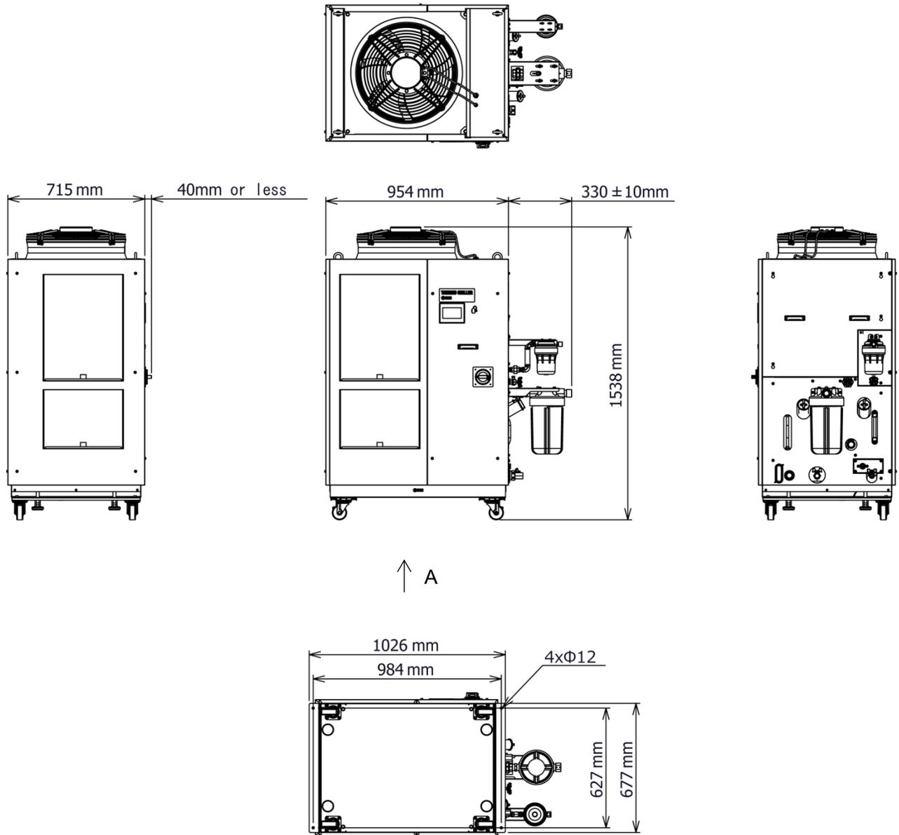
Dimensions for the positions of the anchor bolts (View A)
