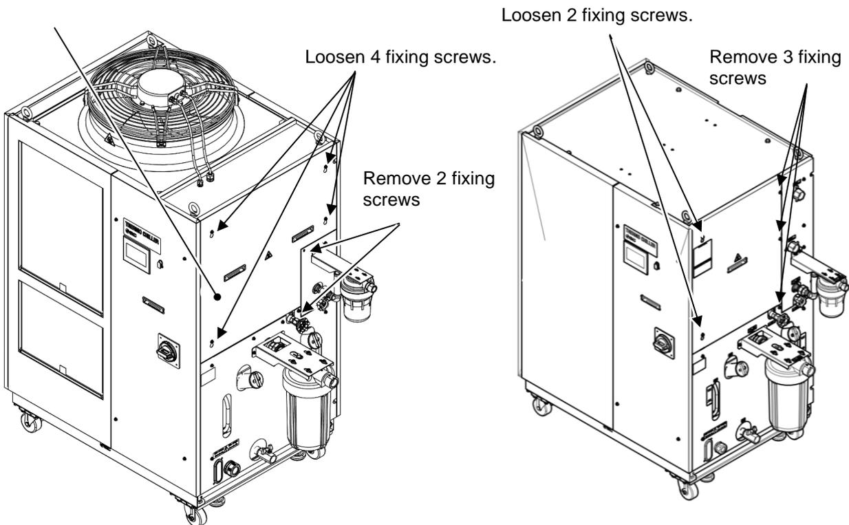
Fig. 7-5 Maintenance panel removal
