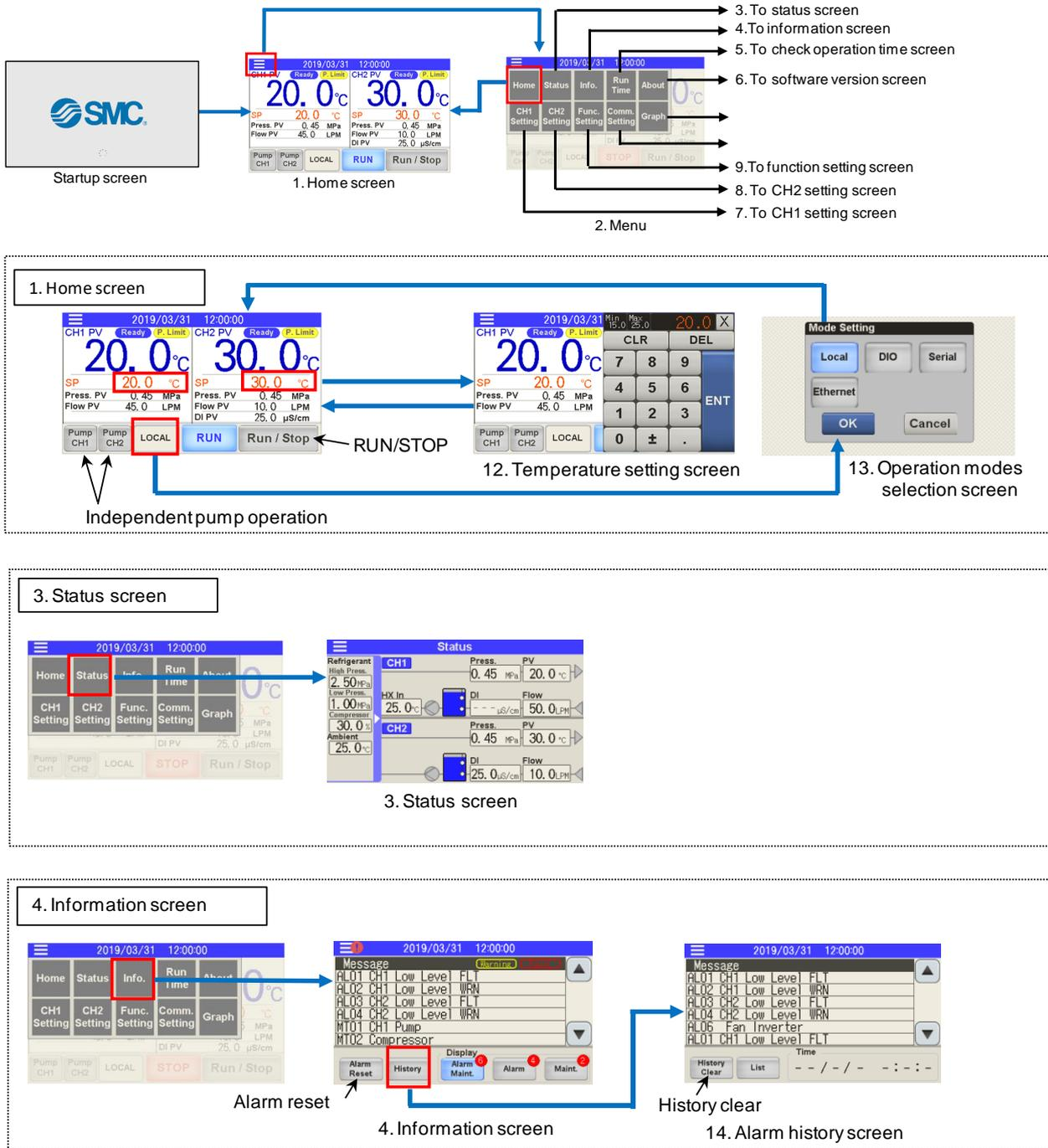
Fig.5-2 Flow chart of operation screen (1/3)
