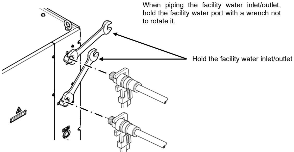
Fig. 3-26 Connection to the facility water inlet/outlet
