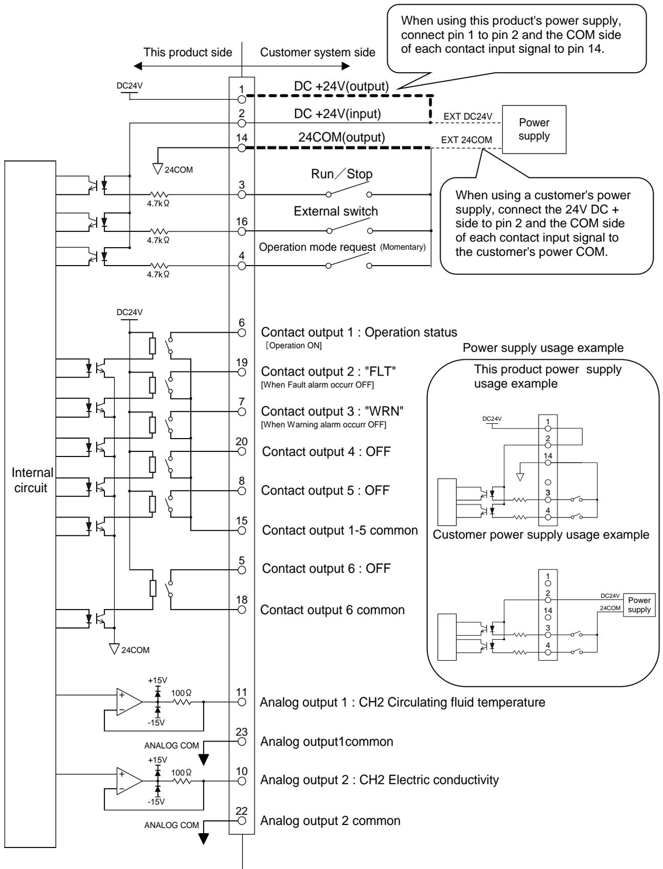
Fig. 3-11 Circuit diagram
