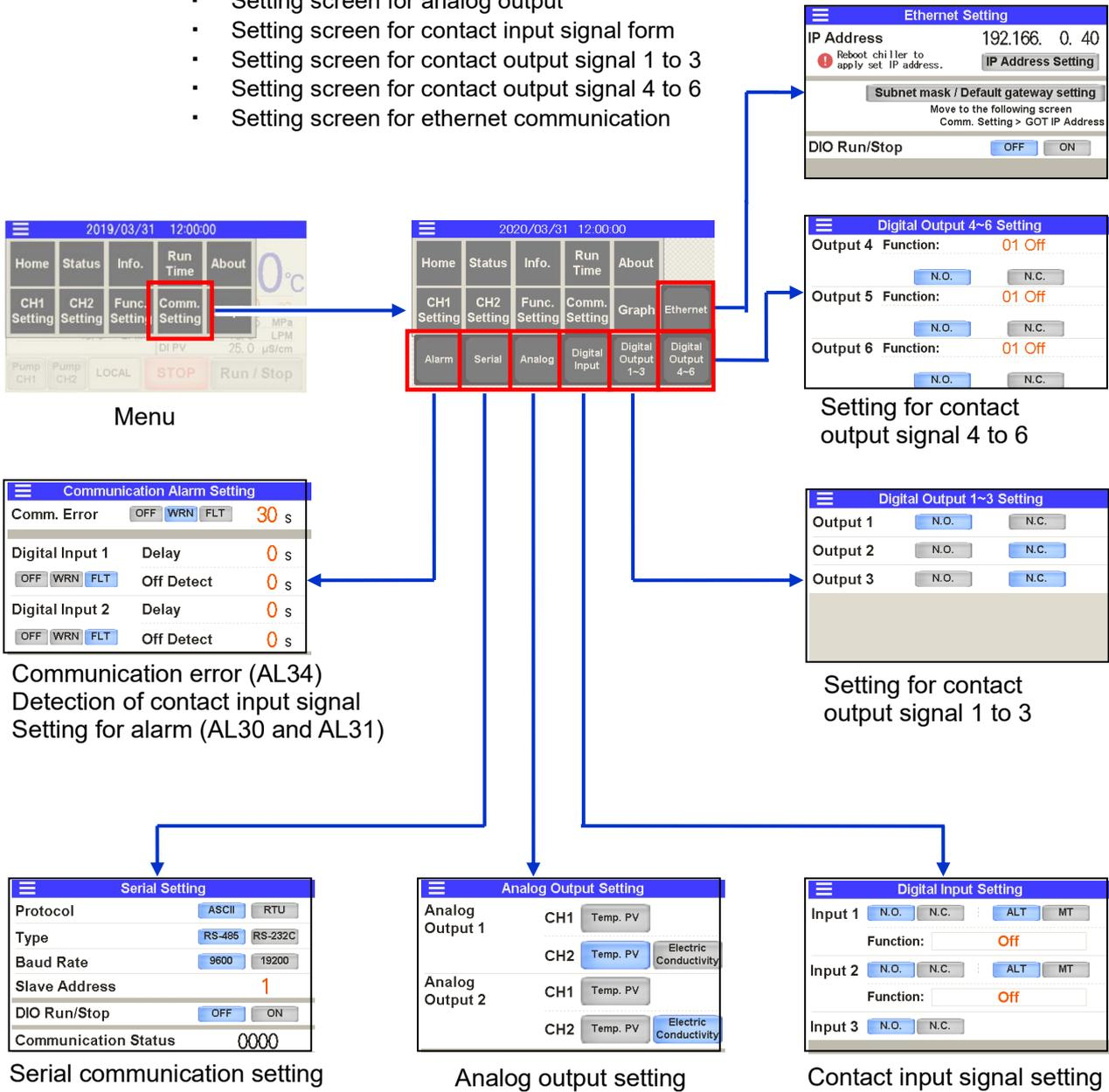
• Setting for communication error (AL34)/contact input signal detection (AL30 and AL31)
