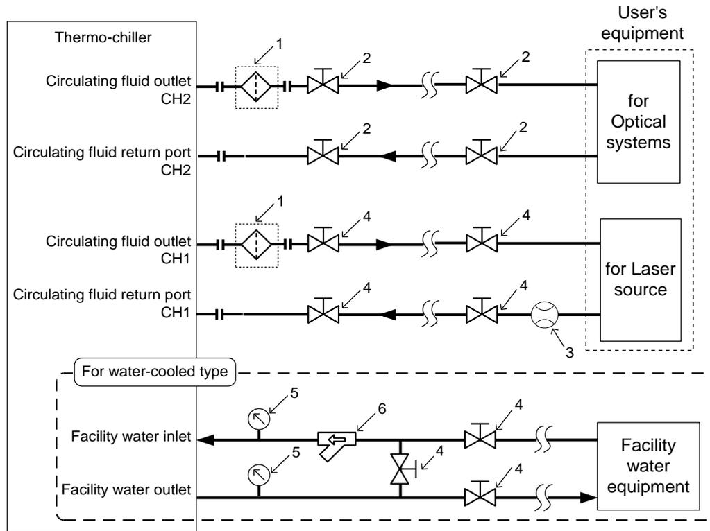
Fig. 3-27 Recommended piping circuit
