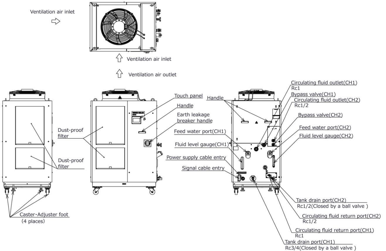
Fig. 2-2 Names of the parts (This drawing shows "HRL200-A-20".)
