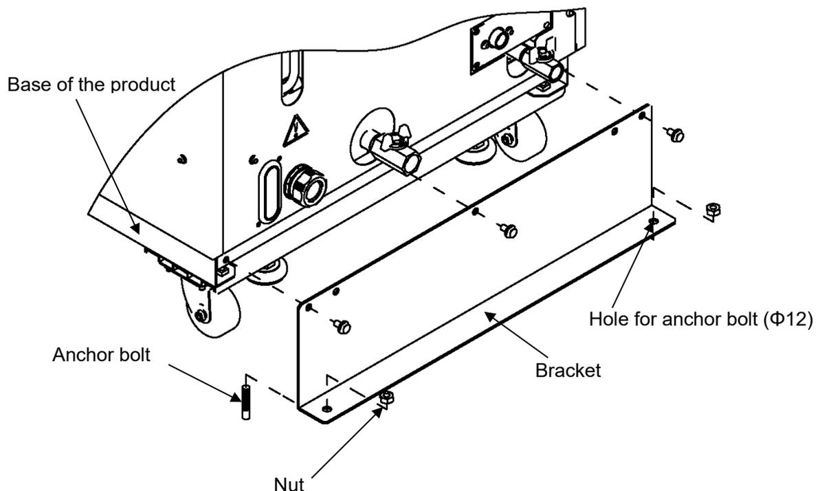
Fig. 3-4 Installation procedures
