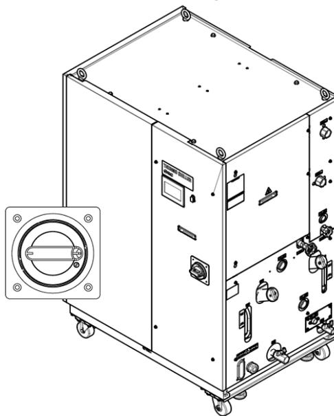
Fig. 3-7 Remove the front panel for the electrical unit (For water-cooled type)
