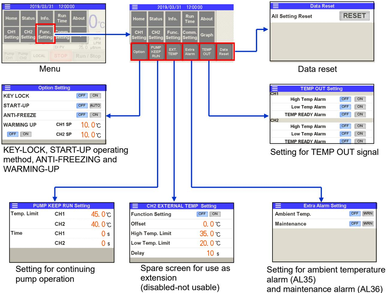
•KEY-LOCK, START-UP operating method, ANTI-FREEZING and WARMING-UP
