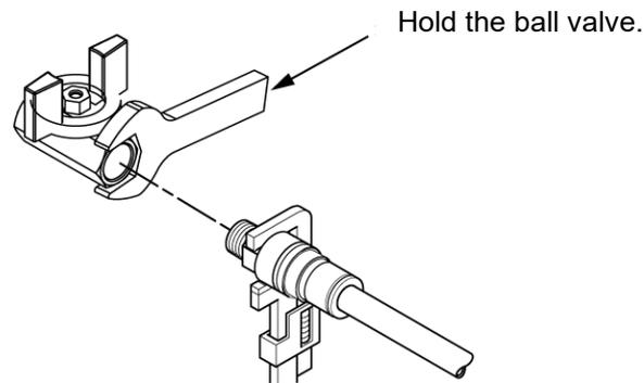
Fig. 3-25 Connection to the drain port
