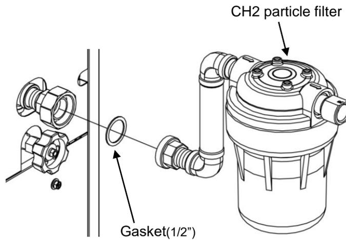
Fig. 3-20 CH2 side Installation of particle filter
