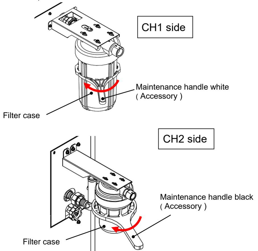
Fig. 7-3 Particle filter removal
