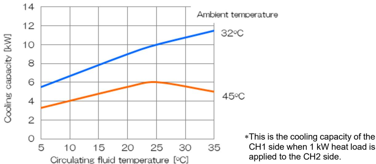
Fig. 8-7 Cooling Capacity (HRL100-A\*-20)
