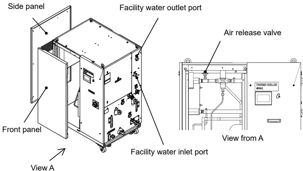
5. After discharging all the facility water, close the air release valve and mount the panel of the electric unit back to the product.
