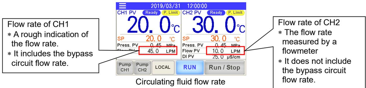
• Circulating fluid flow rate [DI PV]
