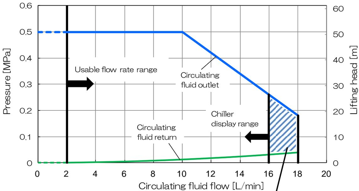
It is available in case of Pressure control mode or Set output mode. However, the Flow rate display of HRL is up to 16L/min.
