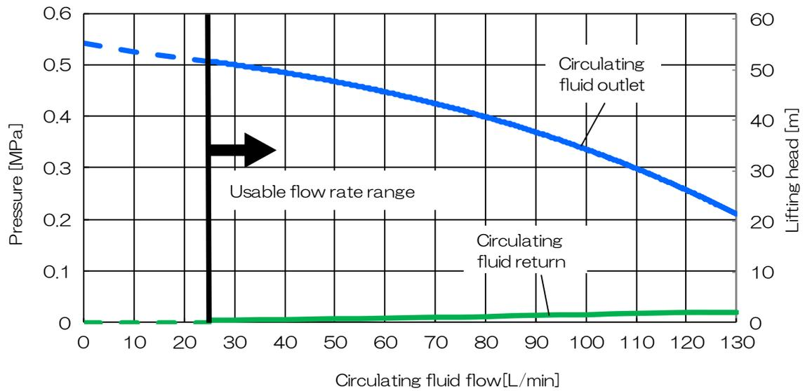
Fig. 8-10 Pump capacity(HRL200-A/W\*-20 CH1)
