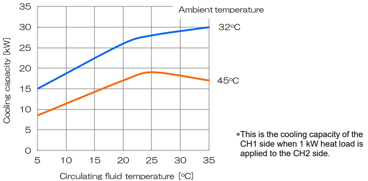
Fig. 8-9 Cooling Capacity (HRL300-A\*-20)
