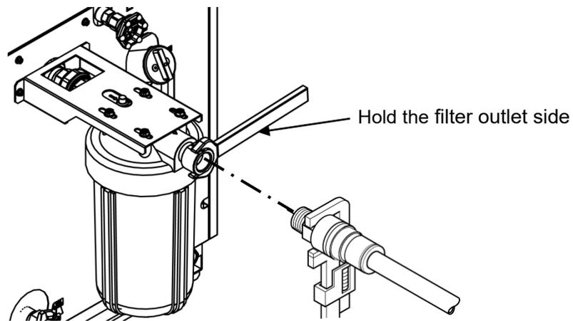
Fig. 3-24 Hold the filter outlet side
