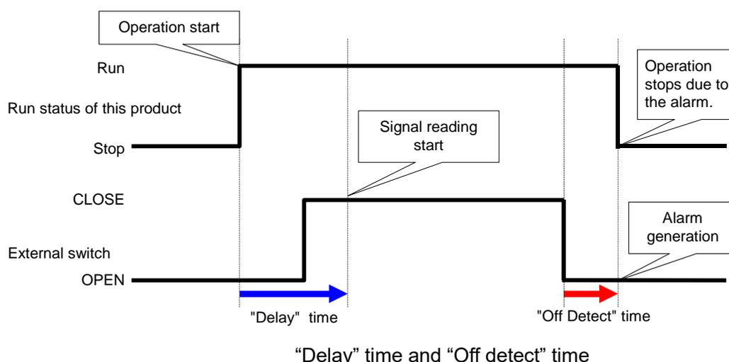
This function is set to “Disabled” by default. Refer to “Setting of contact input signal form” (P.5–57) for details. Contact input signal can be used to perform the “Run/Stop” of the product. Refer to “Setting of contact input signal form” (P.5–57) for the setting method.
