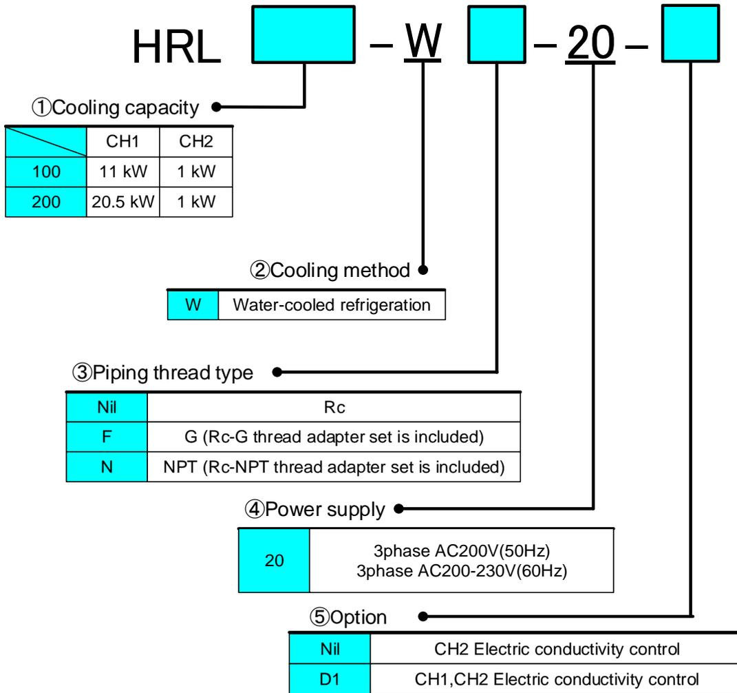
Fig. 2-2 Product model number (Water-cooled type)
