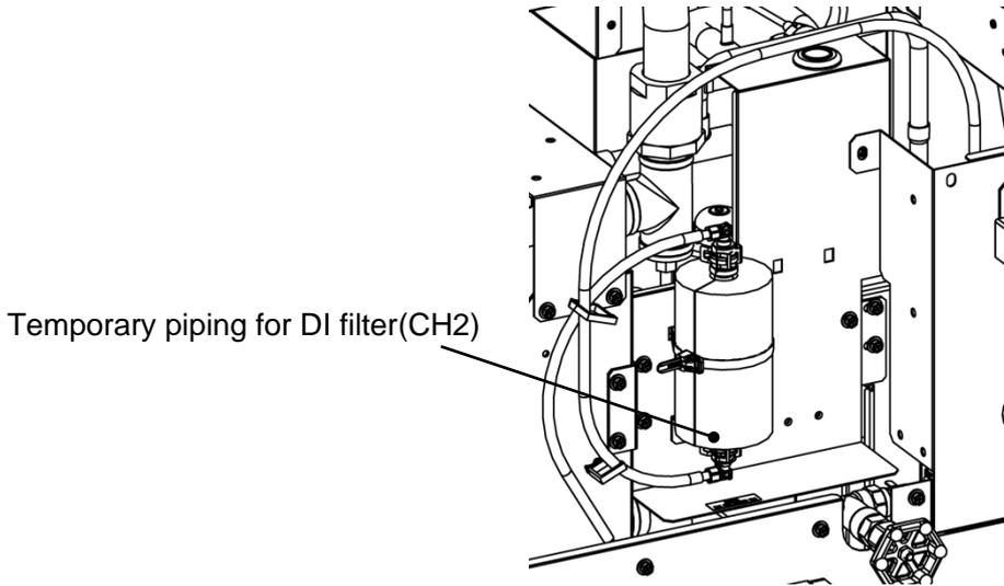
Fig. 8-5 Temporary pipe installation for DI filter
