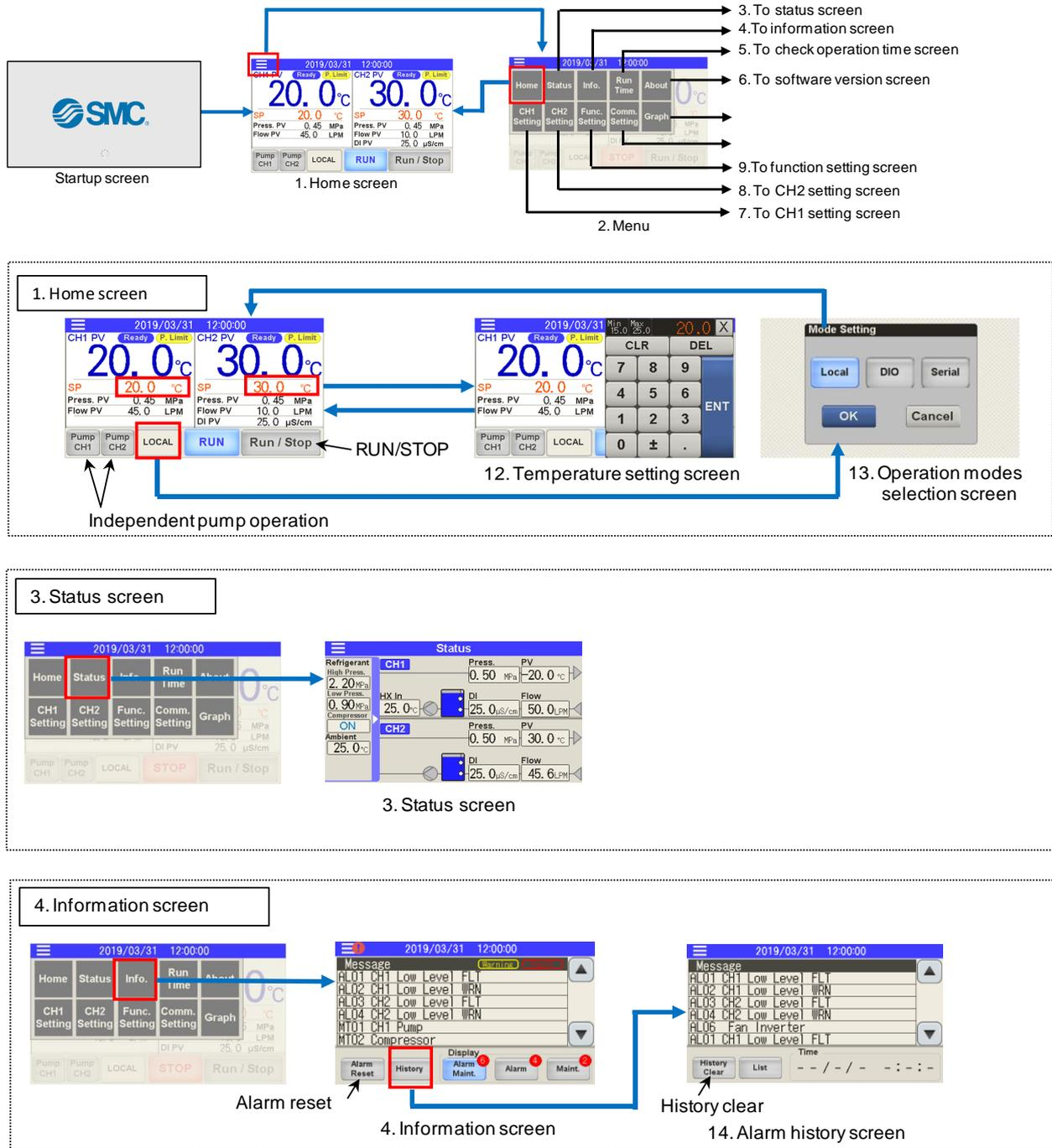
Fig.5-2 Flow chart of operation screen (1/3)
