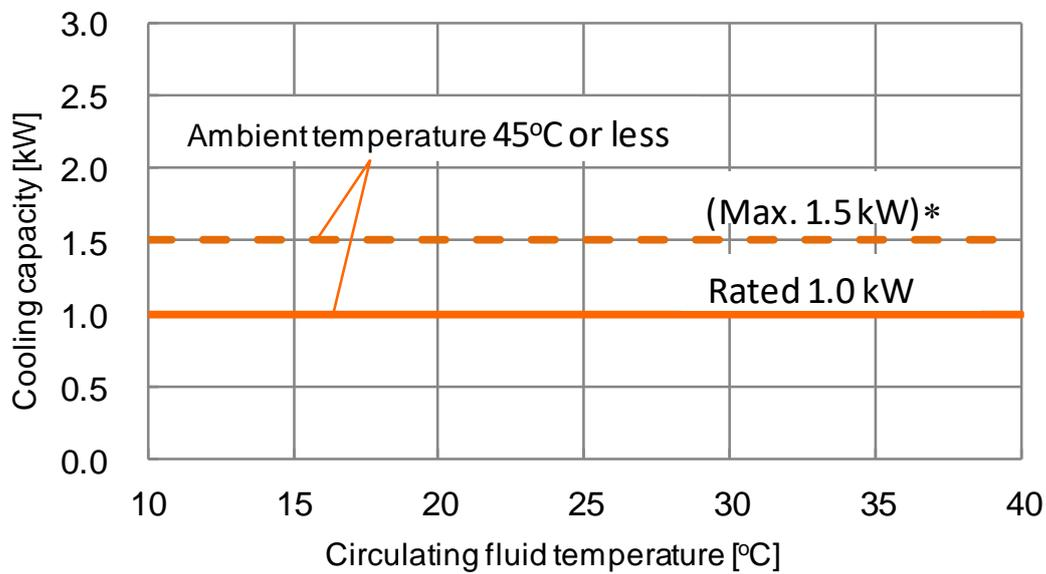
\*Up to 1.5kW. However, when 1.5kW heat load is applied, the cooling capacity of CH1 will decrease by 0.5kW.
