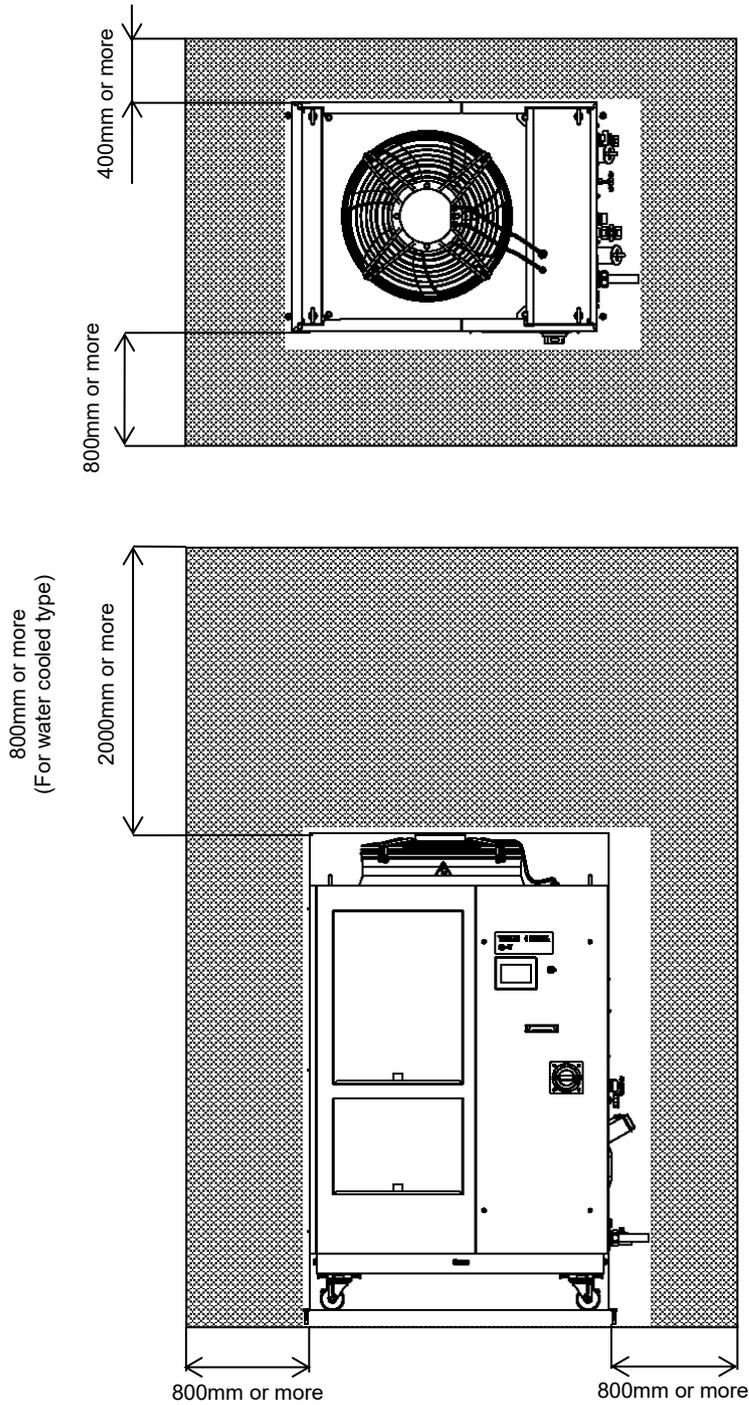
Fig. 3-3 Installation space (This drawing shows “HRL200-A-20”).
