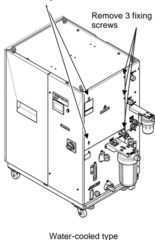
Fig. 8-7 Maintenance panel removal
