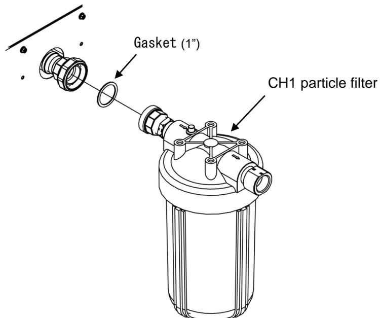
Fig. 3-17 CH1 side Installation of particle filter
