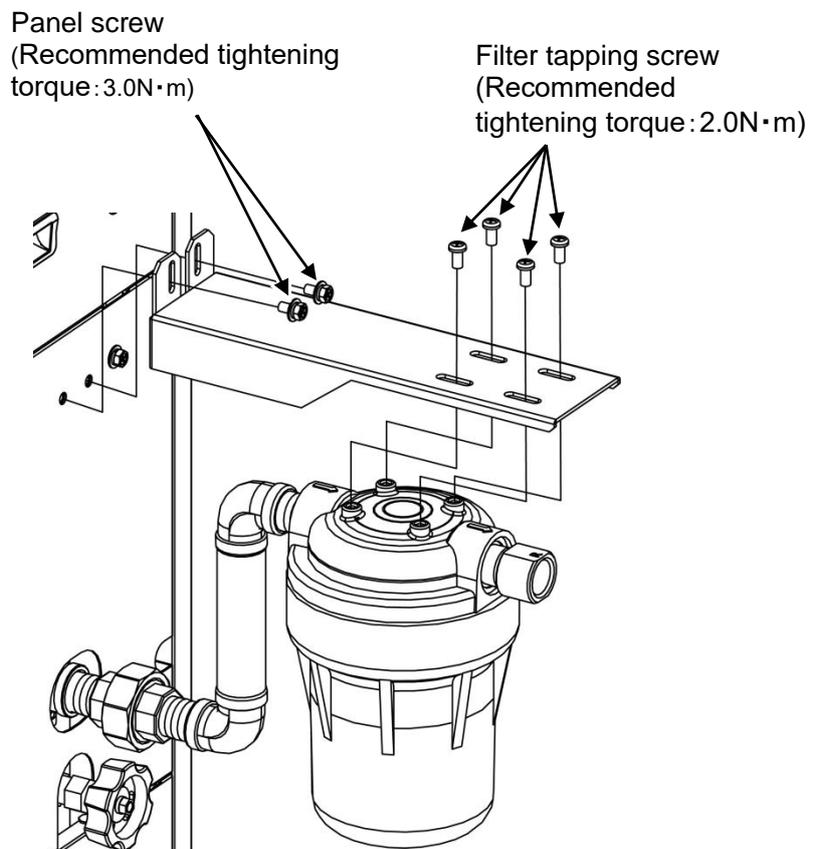
Fig. 3-21 CH2 side Installation of filter bracket.
