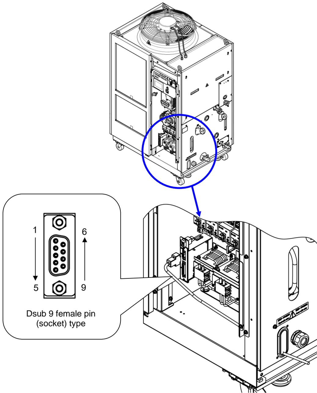
Fig. 3-13 RS-485 communication wiring
