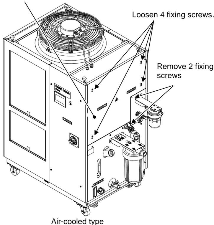
Loosen 2 fixing screws.
