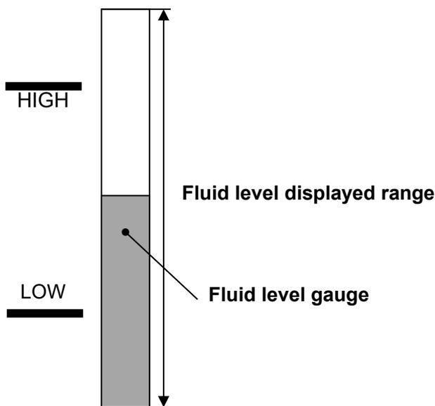
Fig. 3-32 Fluid level gauge
