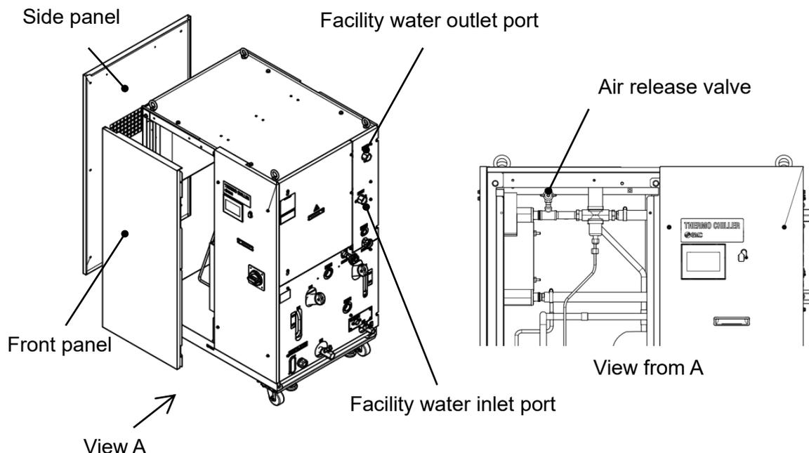
5. After discharging all the facility water, close the air release valve and mount the panel of the electric unit back to the product.
