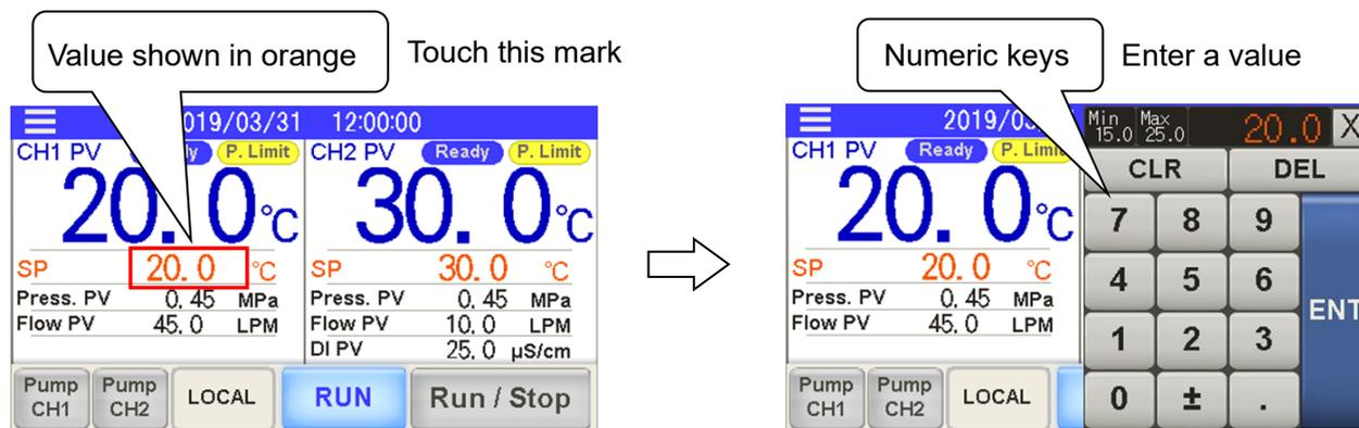
Fig. 4-8 Setting of CH1 circulating fluid temperature
