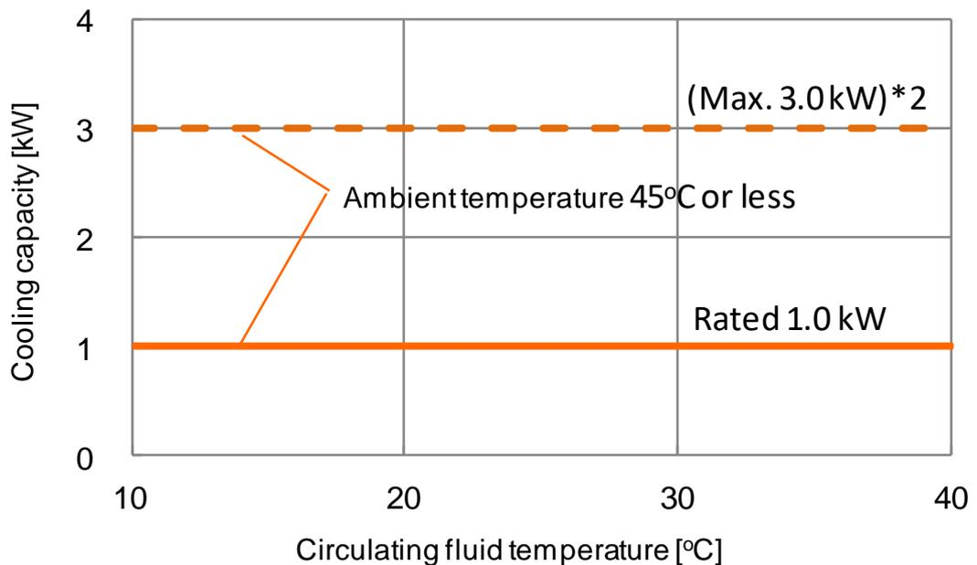
\*Up to 3.0kW. However, when 3.0kW heat load is applied, the cooling capacity of CH1 will decrease by 2.0kW.
