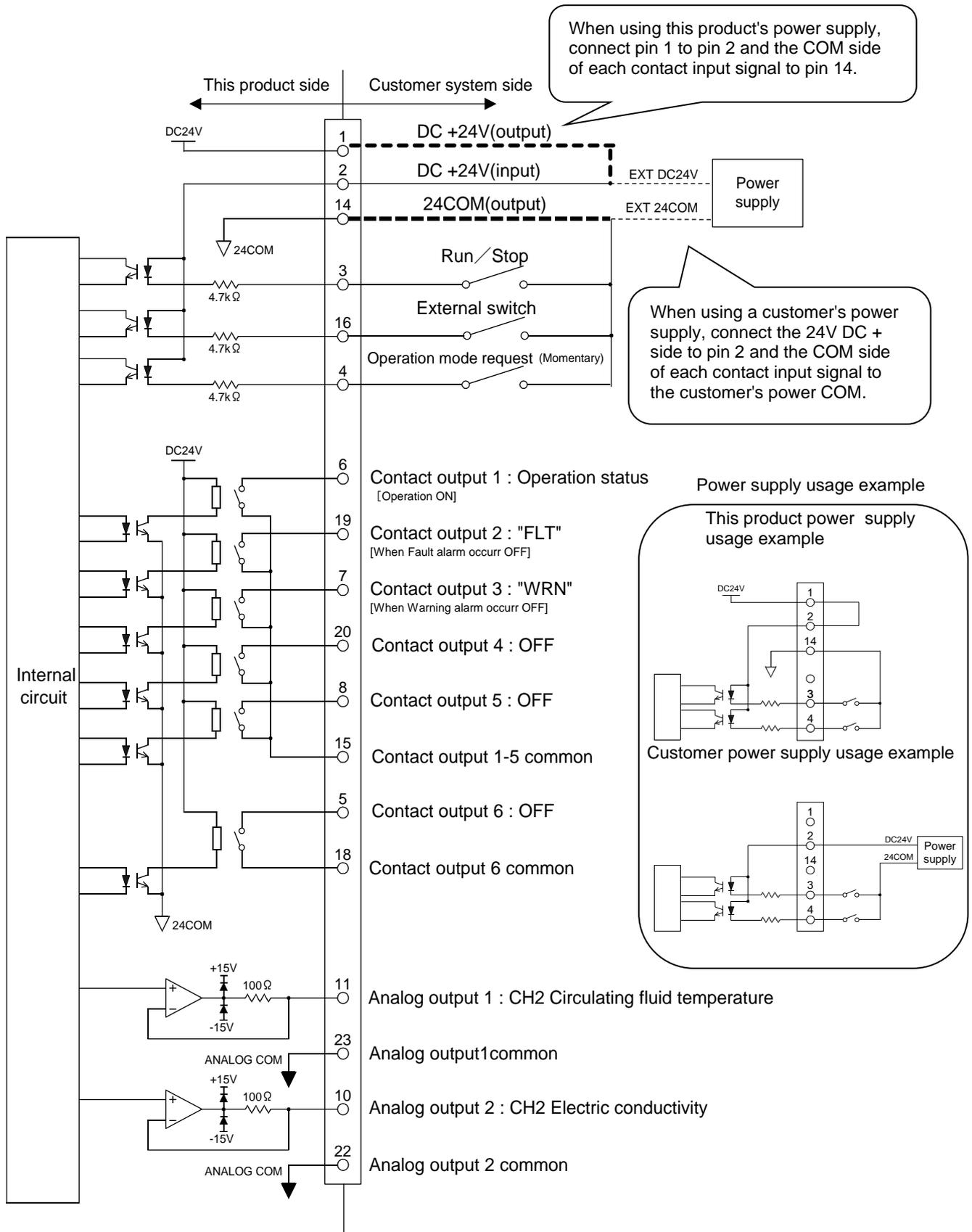
Fig. 3-11 Circuit diagram
