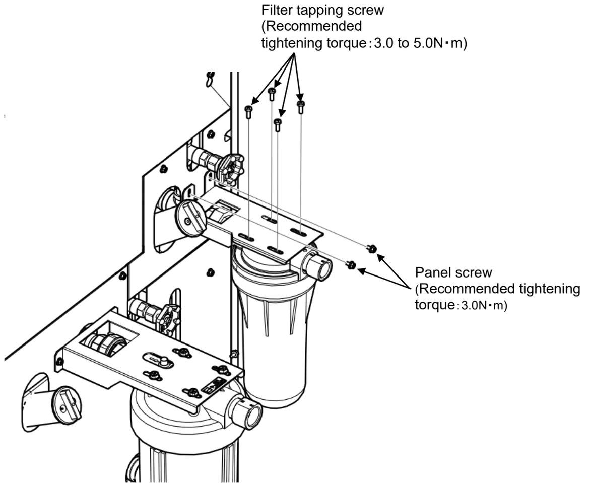
Fig. 3-24 CH2 side Installation of filter bracket.
