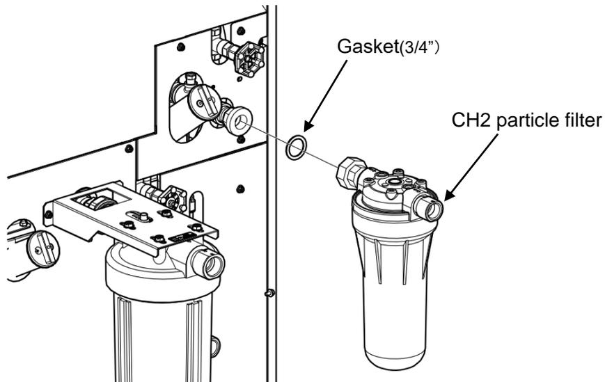
Fig. 3-23 CH2 side Installation of particle filter
