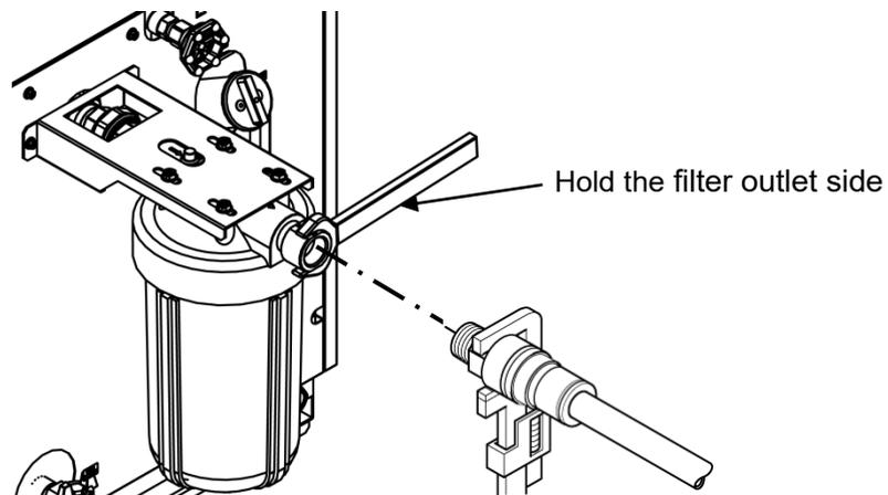
Fig. 3-27 Hold the filter outlet side
