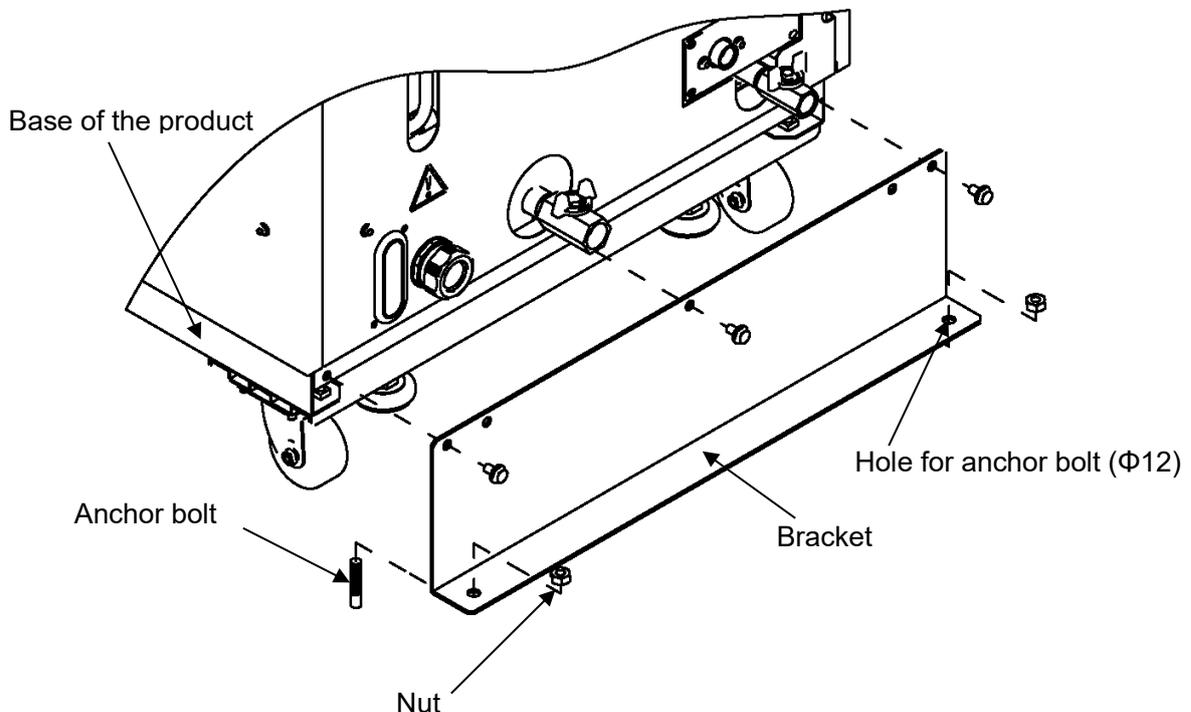
Fig. 3-4 Installation procedures
