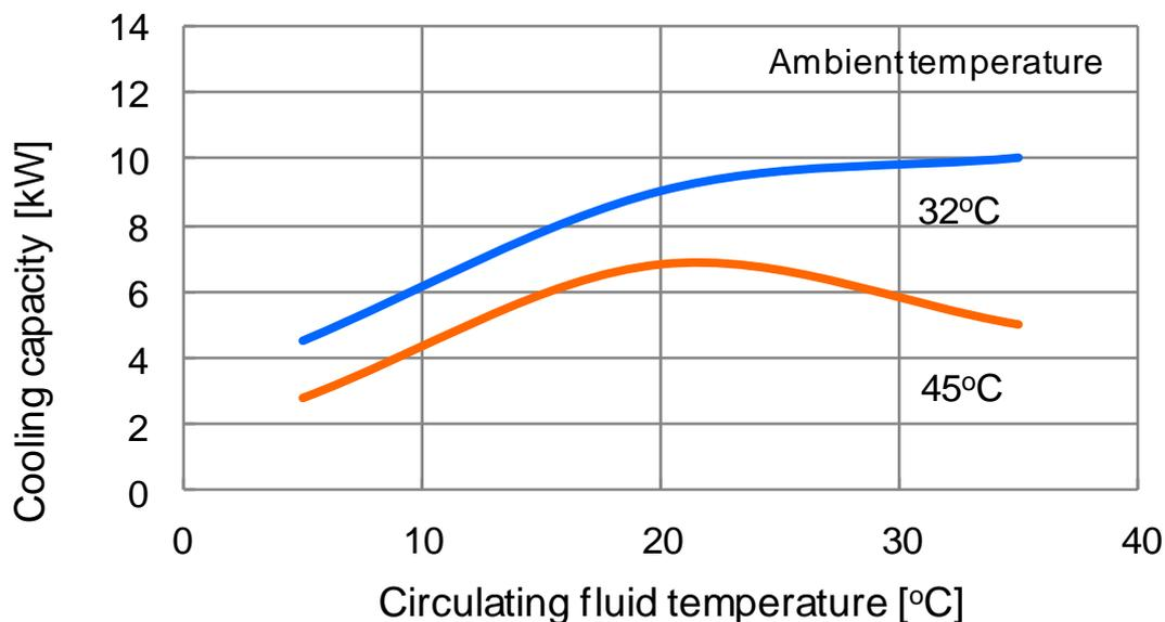
\*This is the cooling capacity of the CH1 side when 1 Kw heat load is applied to the CH2 side.
