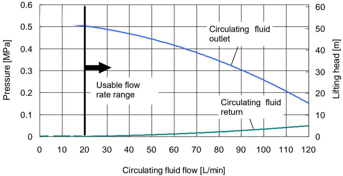
Fig. 9-23 Pump capacity(HRL100-A/W\*-40 CH1)
