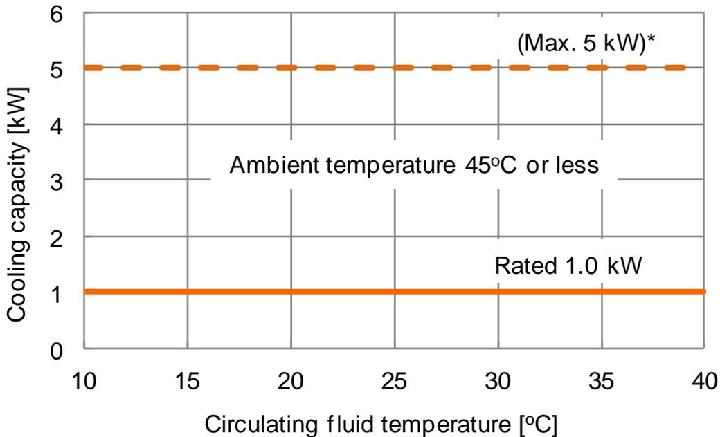
\*Up to 5.0kW. However, when 5.0kW heat load is applied, the cooling capacity of CH1 will decrease by 4.0kW.
