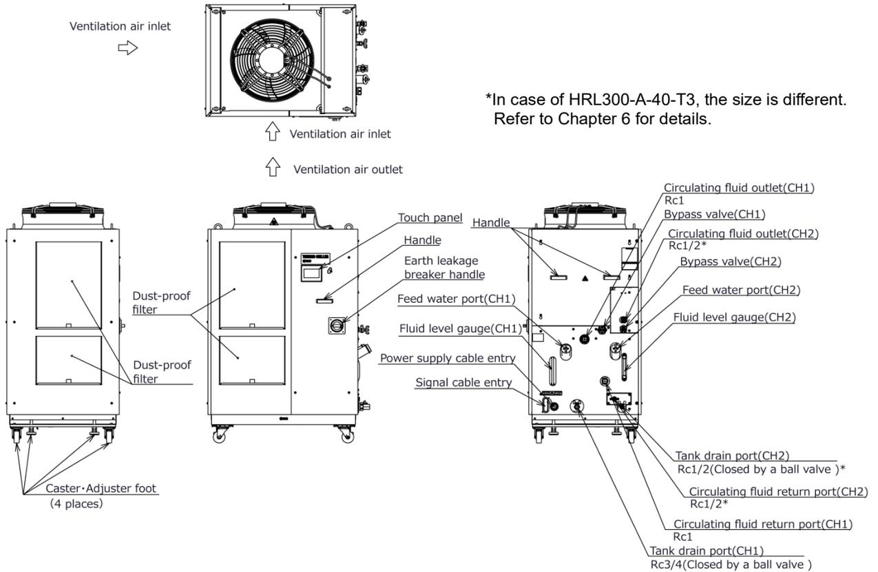
Fig. 2-2 Names of the parts (This drawing shows "HRL200-A-40".)
