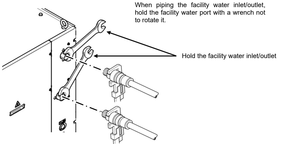
Fig. 3-29 Connection to the facility water inlet/outlet
