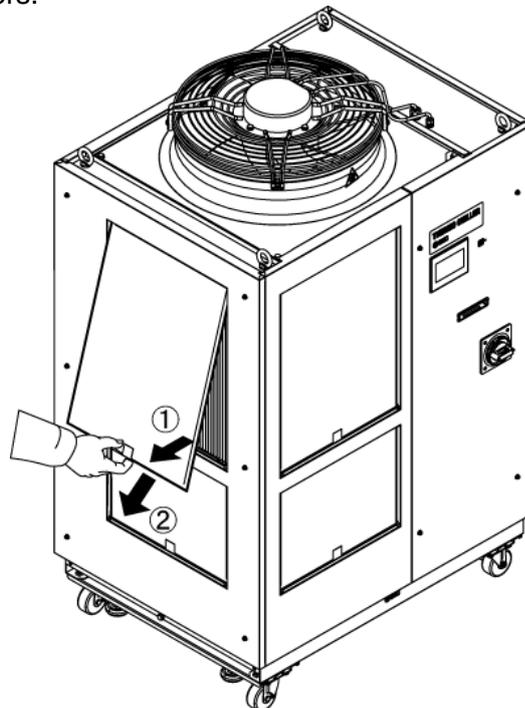
Fig. 8-1 Removal of the dust-proof filter
