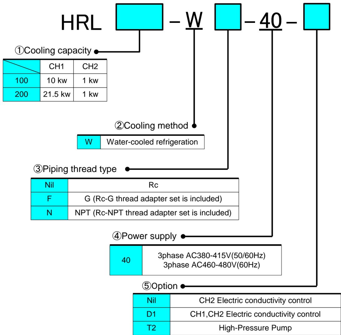
Fig. 2-2 Product model number (Water-cooled type)
