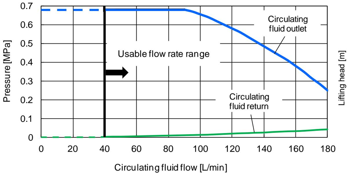
Fig. 9-25 Pump capacity(HRL300-A\*-40 CH1)
