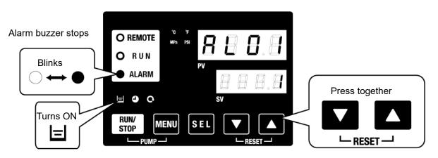
\* []] light turns ON only when "AL01 Low level in tank" alarm is being generated.
