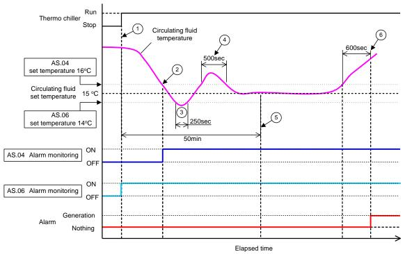
Fig 5.22-2: Alarm generation timing
