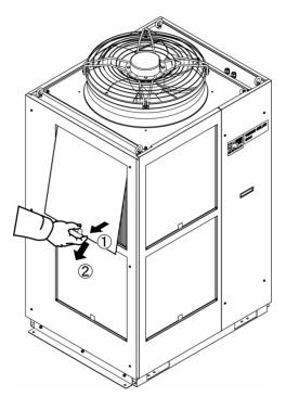
Fig. 7-1: Removal of the dust-proof filter
