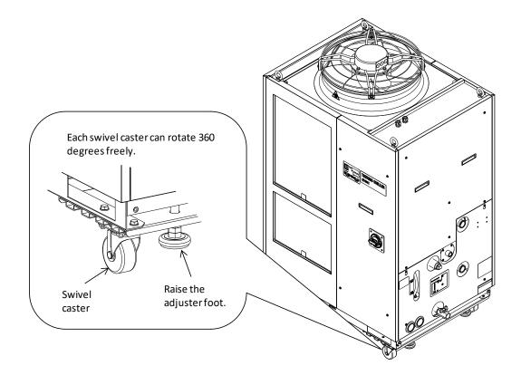
Fig. 3-2 Transportation using casters (This drawing shows "HRSH250-A-20".)
