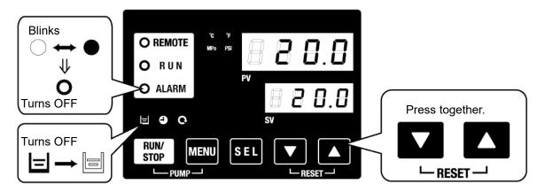
\* [[\_]] light turns ON only when "AL01 Low level in tank" alarm is being generated.
