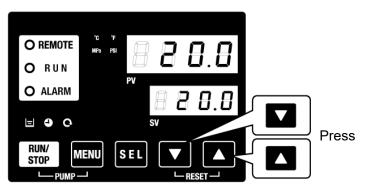
Fig. 4-3 Setting of circulating fluid temperature
