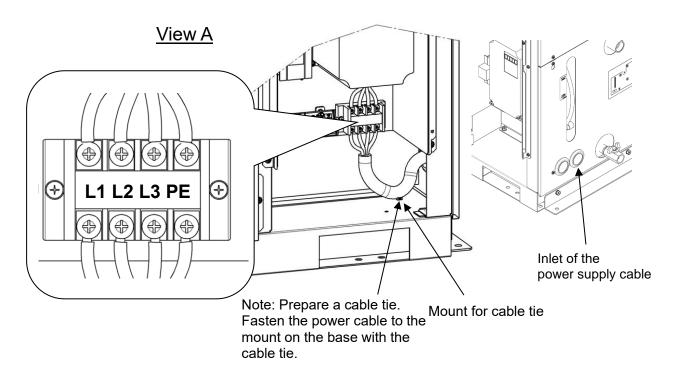
Fig. 3-10 Wiring of power supply cable
