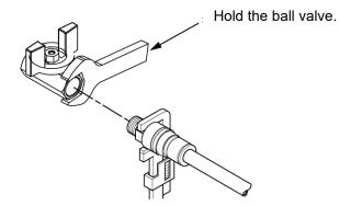
Fig. 3-17 Connection to the drain port
