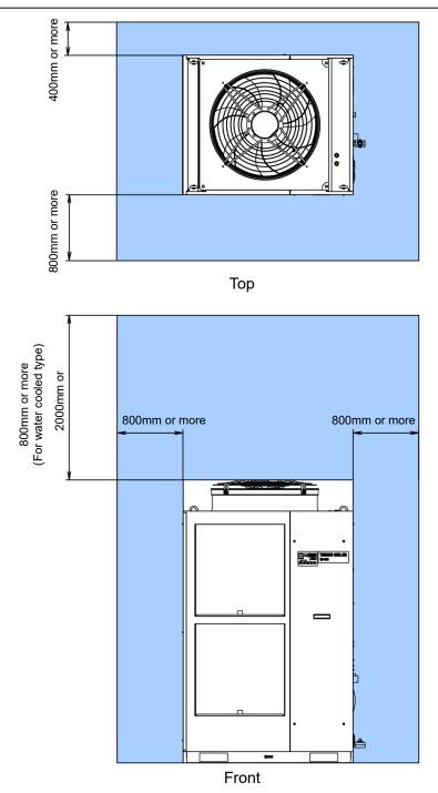
Fig. 3-3 Installation space (This drawing shows "HRSH250-A-20".)
