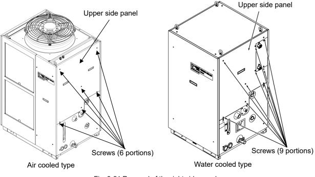
**1.** Remove the screws to remove the upper panel on the right side.
