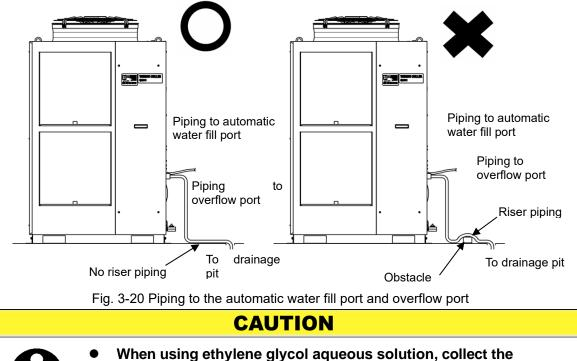
overflowed fluid in the recycling pit and dispose it according to the local law of the country and area that the product is installed.
