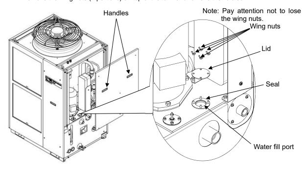
Fig. 3-22 Removal of the right side panel and the lid of the water fill port
