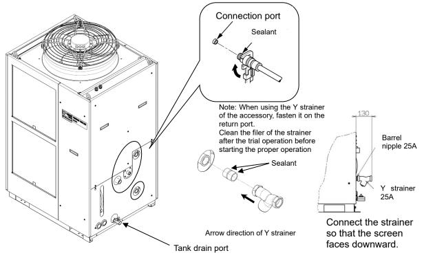
Hold the each piping port with a wrench and tighten the piping.
