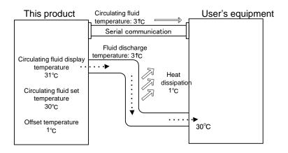
When only the "displayed circulating fluid temperature" needs to be the same as the circulating temperature supplied to the user's equipment:
