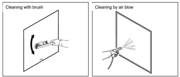
Fig. 7-2: Cleaning of the dust-proof filter
