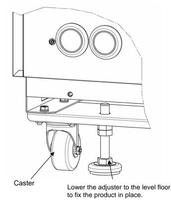
Fig. 3-5 Installation by adjuster foot
