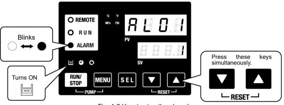
Fig. 4-6 How to stop the alarm buzzer
