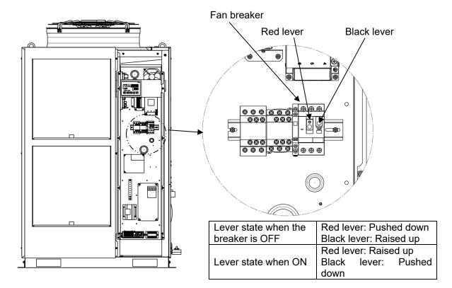
Fig. 6-3: Location and state of the fan breaker
