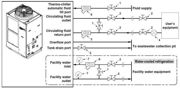
Fig. 3-18 Recommended piping circuit
