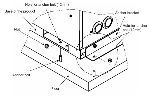
Fig. 3-4 Installation procedures
