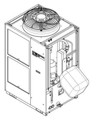
Fig. 3-23 Supplying the fluid to the water fill port (An example)
