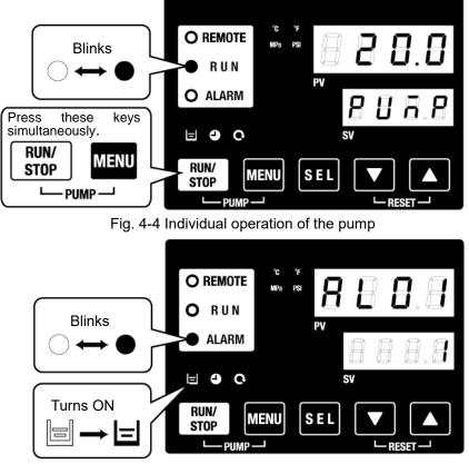
Fig. 4-5 Low level in tank" alarm
