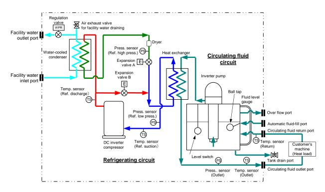
Fig. 8-6: Flow Diagram (HRSH\*\*\*-W\*-20/40-\*)
