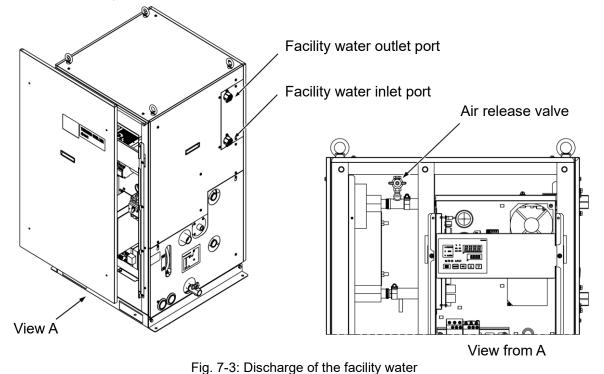
**5.** After discharging all the facility water, close the air release valve and mount the front panel of the electric unit back to the product.
