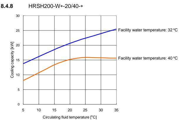
Fig. 8-14: Cooling Capacity (HRSH200-W\*-20/40-\*)
