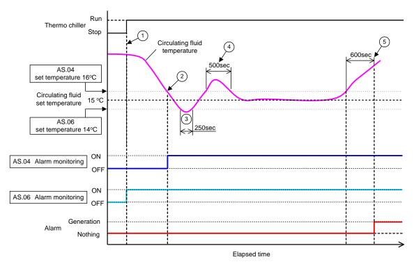
Fig 5.22-1: Alarm generation timing
