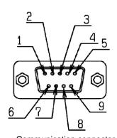
Communication connector D-sub 9 pins (pin type)
