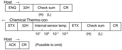
Note) 2DH is entered in 10<sup>1</sup> digit "-" is attached to temperature data.
