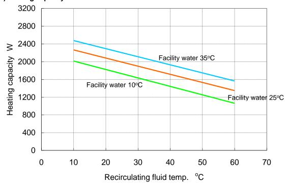
Fig.9-12 Heating capacity (HED007)
