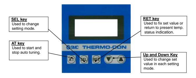
Fig. 5-1 Details of operation panel
