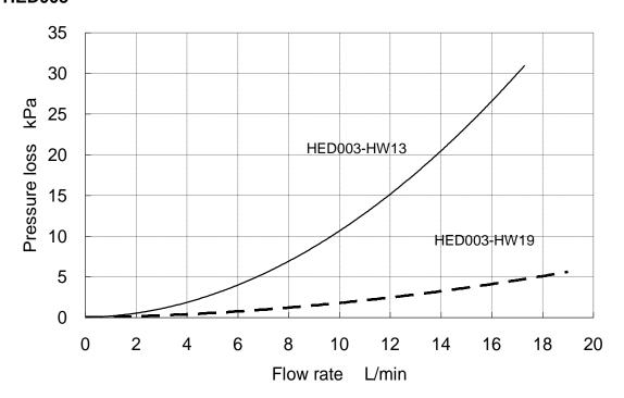
Fig.9-13 Recirculating fluid Pressure loss (HED003)
