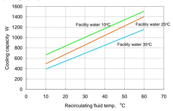
Fig.9-11 Cooling capacity (HED007)
