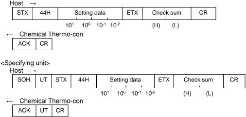
Note) The setting range is from 00.00 to 99.90sec. As 0.1sec is the minimum unit, the number in the hundredths place (10<sup>-2</sup>) should always be 0 (=30H). (When the value at every 0.01sec is input, it is rounded off.)
