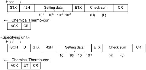
Note) The setting range is from 00.30 to 09.90°C. As 0.1°C is the minimum unit, the number in the hundredths place (10<sup>-2</sup>) should always be 0 (=30H). (When the value at every 0.01°C is input, it is rounded off.)
