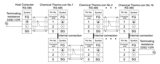
Fig. 7-1 Communication Connection (RS-485)
