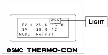
Fig. 6-3 Alarm indication in the event temp. upper and lower limit occurs
