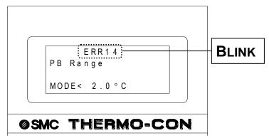
Fig. 6-2 Alarm indication in the event ERR14 occurs during PB range setting input
