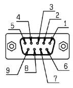
Communication connector D-sub 9 pins (socket type)
