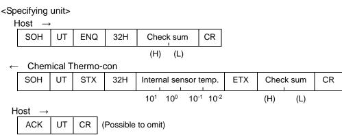
Note) 2DH is entered in 101 digit "-" is attached to temperature data.
