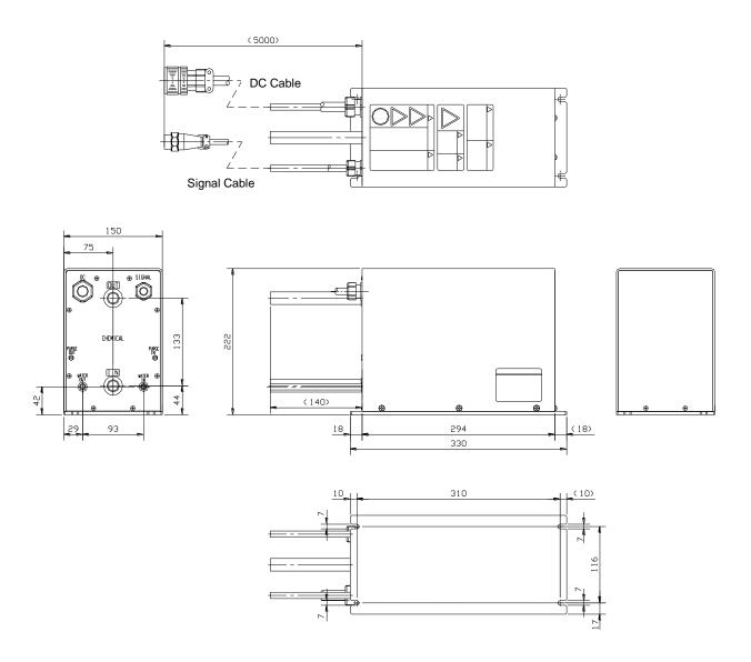
Fig. 9-6 Heat Exchanger
