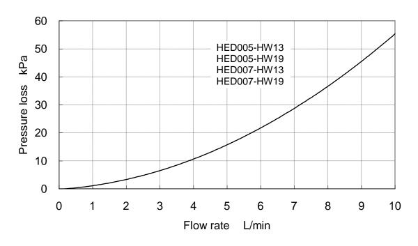
Fig.9-16 Facility water Pressure Loss (HED005/007)
