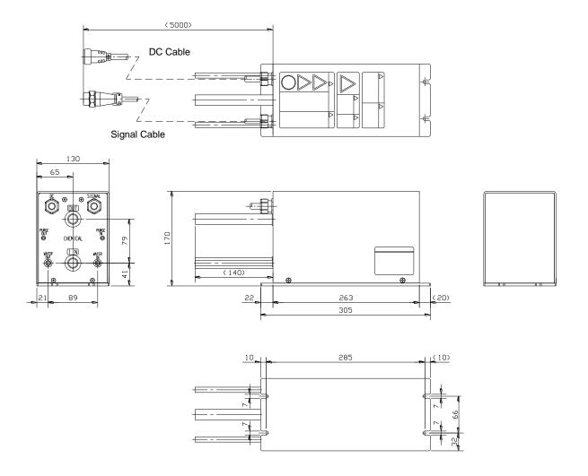
Fig. 9-2 Heat Exchanger
