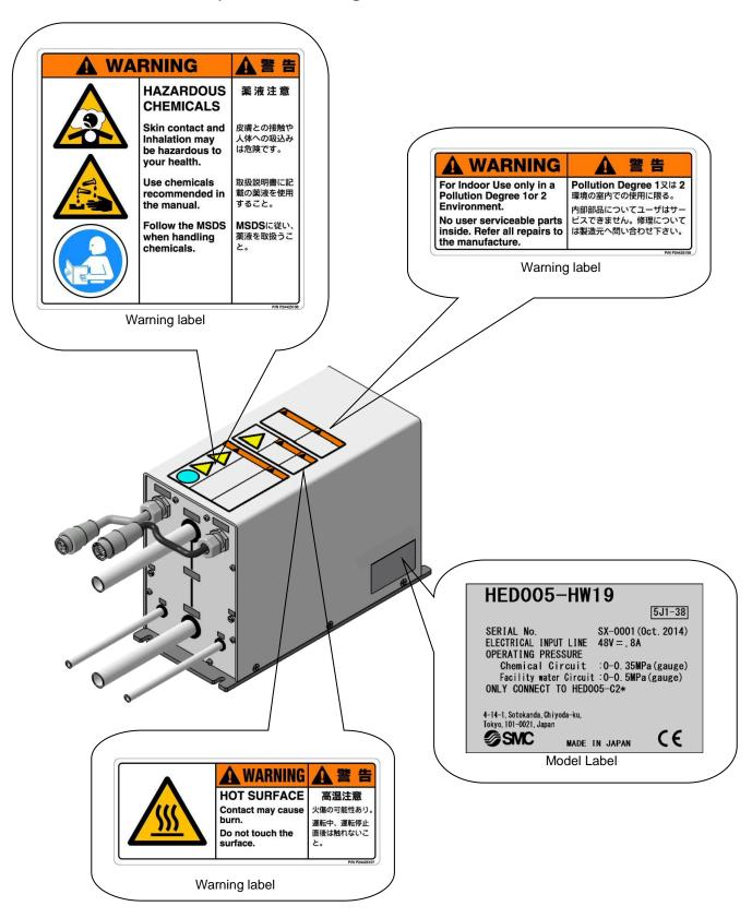
Fig. 1-4 Heat Exchanger
