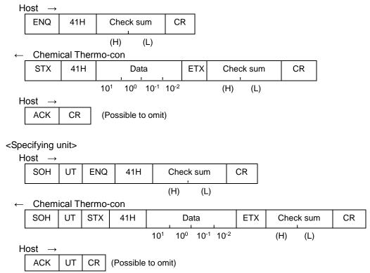
Note) As 0.1°C is the minimum unit, the number in the hundredths place (10<sup>-2</sup>) is always 0 (=30H).
