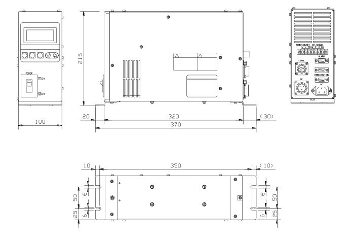
Fig. 9-1 Temperature Controller
