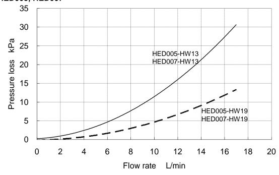
Fig.9-14 Recirculating fluid Pressure loss (HED005/007)
