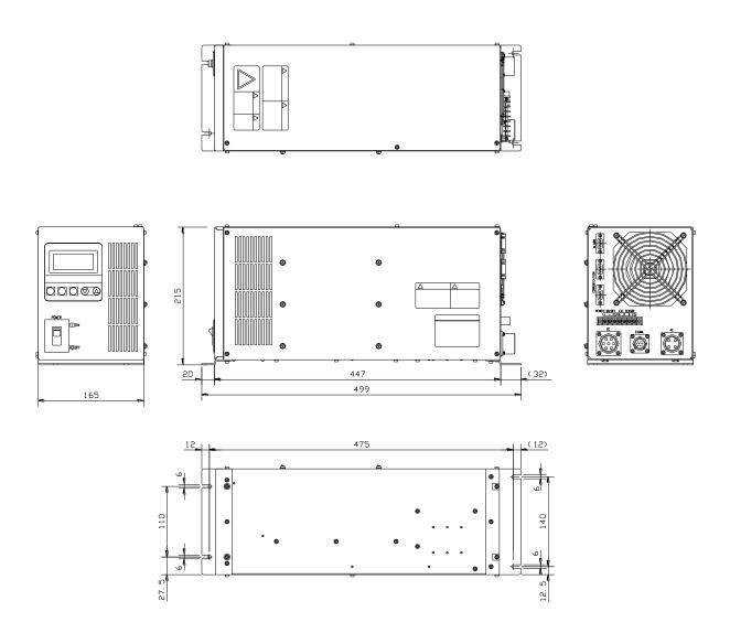
Fig. 9-5 Temperature Controller
