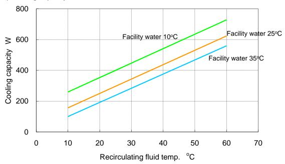
Fig. 9-7 Cooling capacity (HED003)
