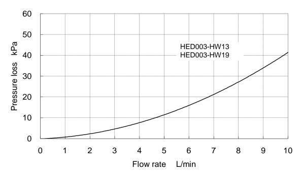
Fig.9-15 Facility water Pressure Loss (HED003)
