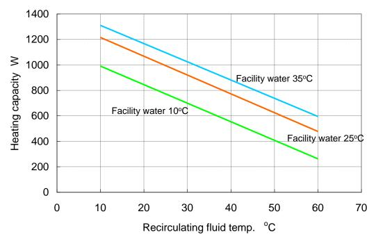
Fig.9-10 Heating capacity (HED005)
