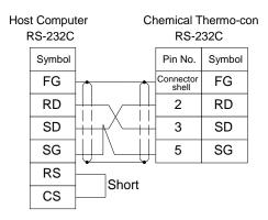
Fig. 7-2 Communication Connection (RS-232C)
