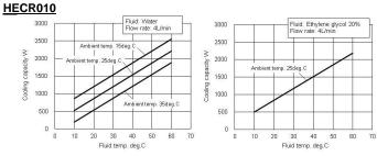
\*Cooling capacity decrease about 50W when high head pump option selected.
