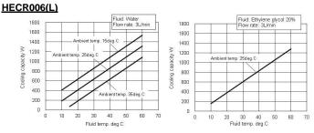
\*Cooling capacity decrease about 50W when high head pump option selected.
