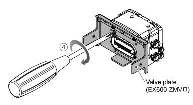
(5) Connect the SI unit and the valve manifold.
