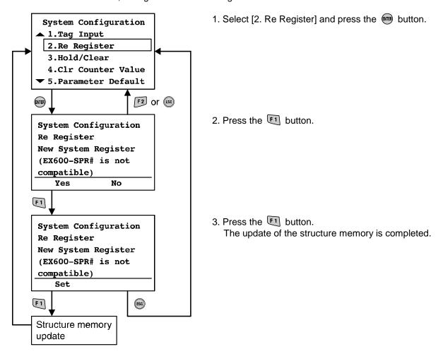
\*1: PROFIBUS DP compatible SI unit is not applicable to memory structure.
