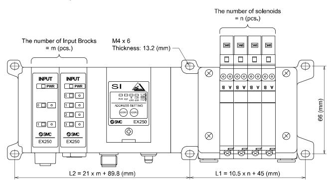
Dimensions when VQC2000 series solenoid valve manifold is connected are shown in the table below for reference.
