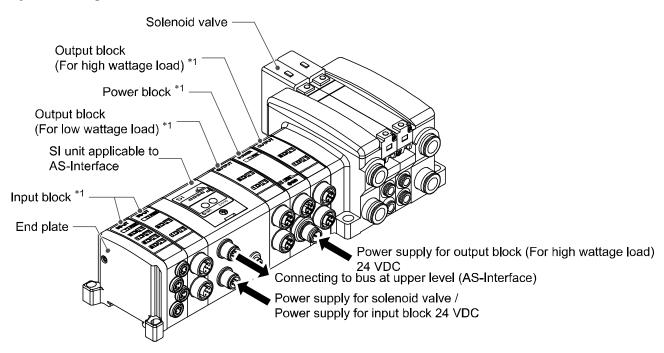
This system connects input/output devices to AS-Interface with reduced wiring. AS-Interface communicates with the input/output devices via the SI unit.
