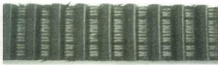
Bottom portion of belt gear worn-out (frayed thread exposed )
