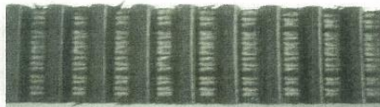
ベルト歯底摩耗（心線露出） Bottom portion of belt gear worn-out (frayed thread exposed)
