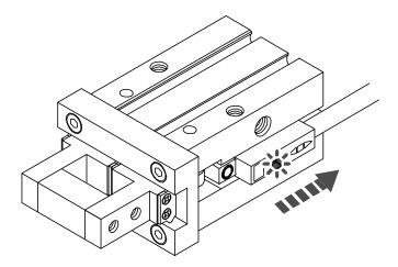
(4) Make sure that the indicator light (READY) on the amplifier unit is ON.
