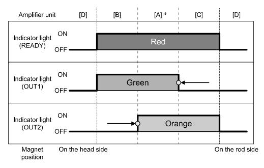
$<sup>\</sup>ast$ : The dimension for [A] should be 0.5 mm minimum in the stroke direction.
