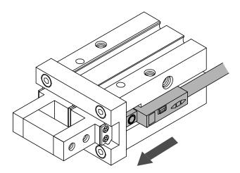
\*: The relationship between OUT1 and OUT2 is reversed if the mounting direction is opposite. The Detection range may change. An Operation check with actual equipment should be performed as the location of OUT1 and OUT2 is reversed depending on the air gripper structure. (3) Pull back the sensor unit. Position the sensor unit where the indicator light changes from red to green.
