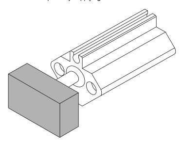
(2) Insert the sensor unit up to the end of the mounting groove. (Figure below) \*
