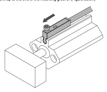
\*: The relationship between OUT1 and OUT2 is reversed if the mounting direction is opposite. The Detection range may change. An Operation check with actual equipment should be performed as the location of OUT1 and OUT2 is reversed depending on the cylinder structure.
