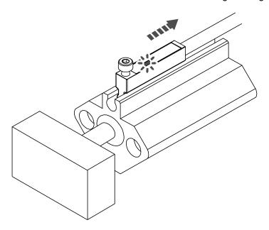
(4) Make sure that the indicator light (READY) on the amplifier unit is ON.
