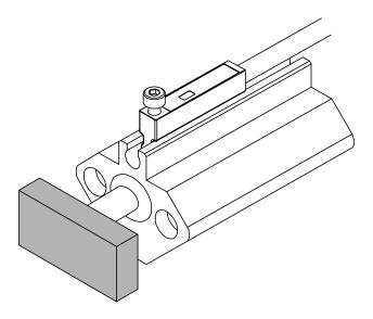
(8) Turn the adjustment trimmer (OUT2) with a screwdriver. Stop turning the screwdriver when the indicator light (OUT2) is ON.
