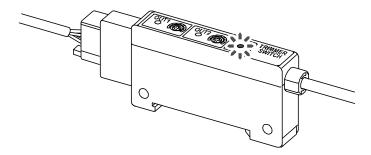
(5) Fix the sensor unit using the mounting screw or a mounting bracket. Refer to the table below for the tightening torque.
