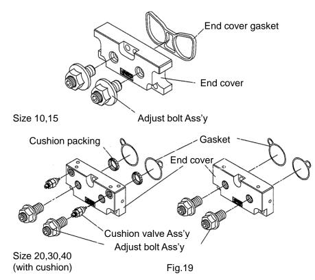
Insert and attach the cushion packing and the packing with the direction in the drawing below.
