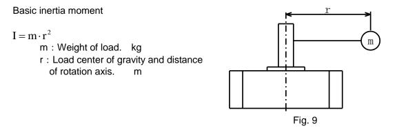
This shows inertia moment of "m (weight)" at "r" from the rotation axis. Calculation of inertia moment depends on the shape of the object. Please refer the table on the next page for inertia moment calculation.
