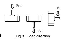
\*Point of application of force of Fr is the center of shaft flat face and longer dimension of the key.
