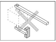
If an external stopper is installed on the opposite side of the load, the inertia force generated by the load is applied directly to the table.
