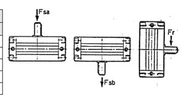
Point of application of force of Fr is the center of shaft flat face and longer dimension of the key.
