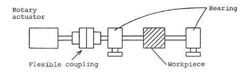
Fig. (6) Flexible coupling
