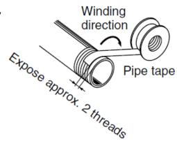
Fig. (9) Wrapping of pipe tape
