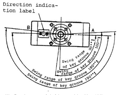
Fig. (2) Rotation range of shaft keyway (size 50 to 100)
