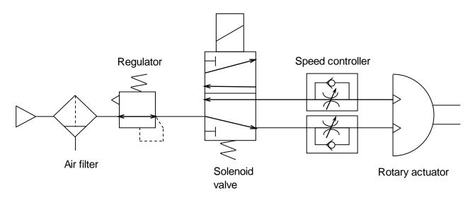
Fig. (3) Basic circuit
