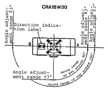
Stopper screw A: For end adjustment in clockwise direction
