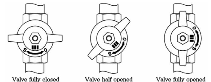
【The relationship between the opening of the valve of the standard pump / by-pass piping and the guide for the flow rate】
