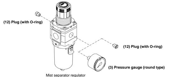
12-3. Disassembly Drawing of the Pressure Gauge Port [Applicable model: with square embedded type pressure gauge / with digital pressure switch]
