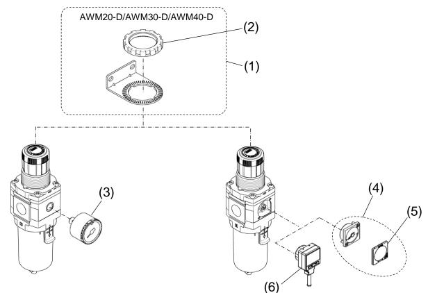
Without pressure gauge/ With round type pressure gauge With square embedded type pressure gauge/ With digital pressure switch
