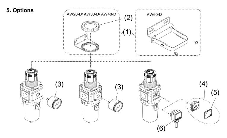
Without pressure gauge/ With round type pressure gauge (Backflow function: No) Without pressure gauge/ With round type pressure gauge (Backflow function: Yes) With square embedded type pressure gauge/ With digital pressure switch (Backflow function: No / Yes)
