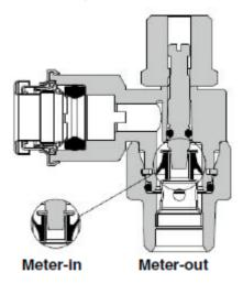
Seal method: Face seal For G thread
