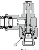
Seal method: Sealant For R, NPT thread
