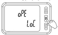
(2) Select the un-locking [UnL] using the UP or DOWN button. Setting is recognized by pressing the SET button, then the security code is required. When the security code is set, select the un-lock [UnLoC] using the UP or DOWN button. Setting is recognized by pressing the SET button, then the security code is required. If the security code is not set, select the un-lock [UnLoC]. Locking is released by pressing the SET button.
