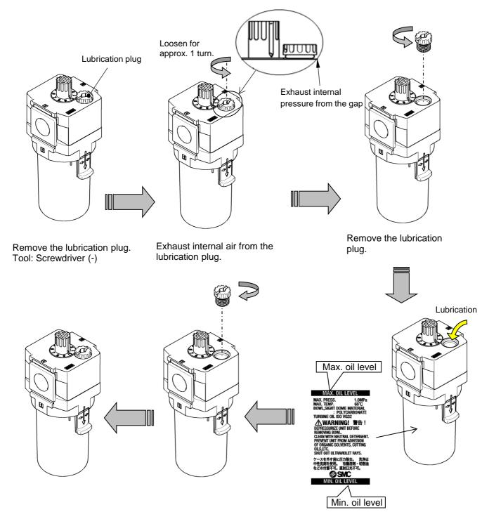
After supplying lubricant, check the mounting condition of the lubrication plug O-ring and screw it in gently.
