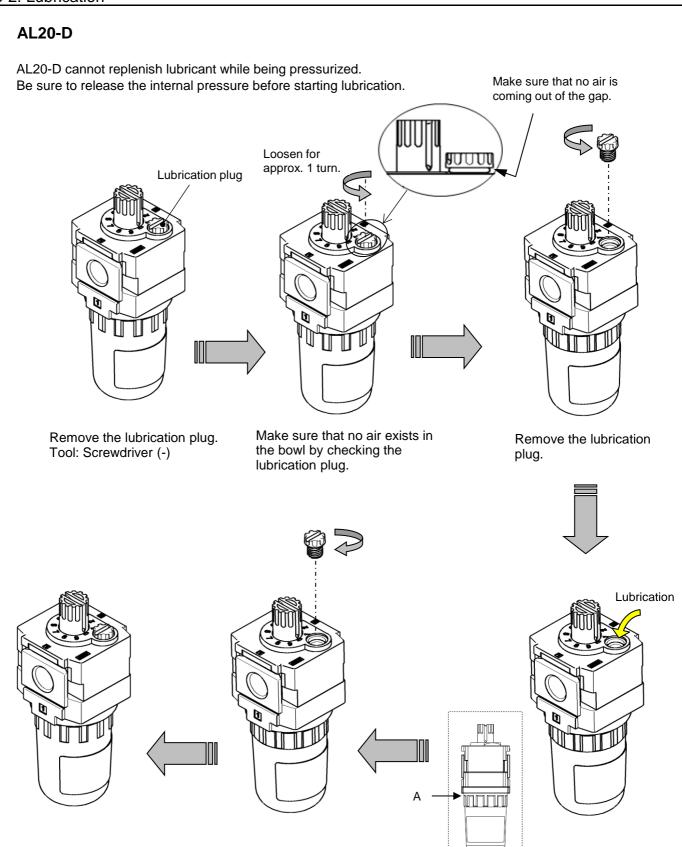
After supplying lubricant, check the mounting condition of the lubrication plug O-ring and screw it in gently.
