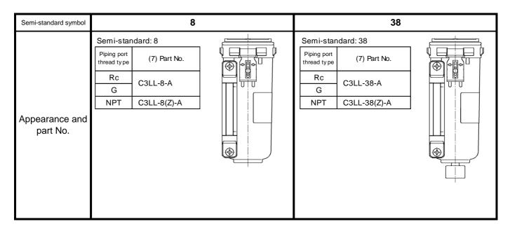
Note 1) Part No. (7) includes Bowl seal (6). Refer to section [11. Disassembly Drawing] (P31).
