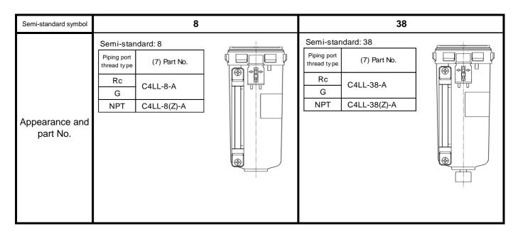
Note 1) Part No. (7) includes Bowl seal (6). Refer to section [11. Disassembly Drawing] (P31-32).
