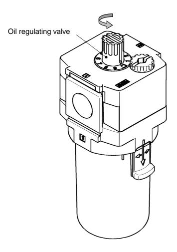
While supplying air, rotate the oil regulating valve to adjust the amount of oil.
