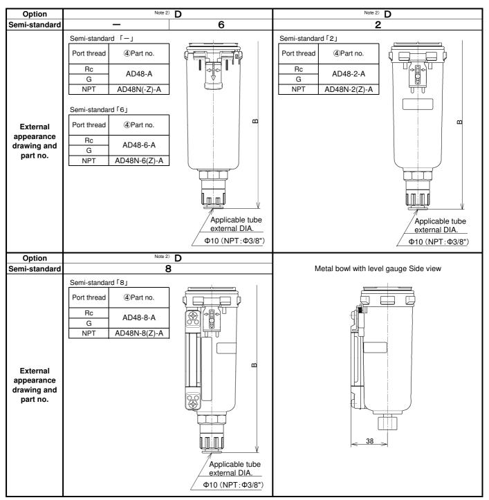
Note 1) B in the table shows the distance from inlet piping centreline to drain port. Refer to "12. DIMENTIONS" (P24).
