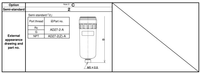
Note 1) B in the table shows the distance from inlet piping centreline to drain port. Refer to "12. DIMENTIONS" (P24). Note 2) Min. operating pressure is 0.1MPa.
