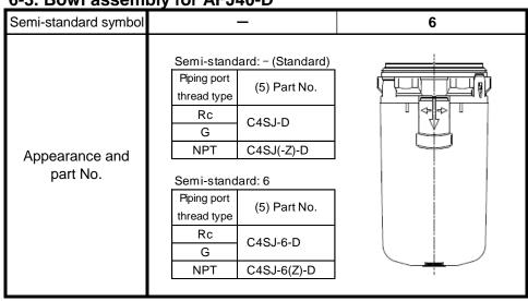
Note 1) Part No. (5) includes Bowl seal (4). Refer to the section [10. Disassembly Drawing] (P17).
