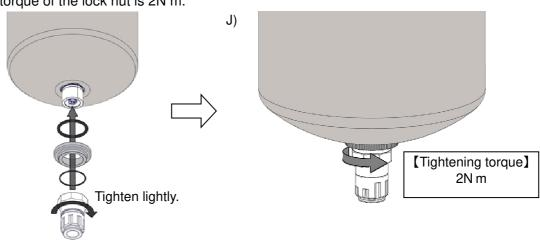
K) Insert the guide and element in order, and mount the O-ring for the bowl.If the support ring was removed, mount the support ring before the O-ring for bowl.Note: Ensure that the element inserting direction is correct.
