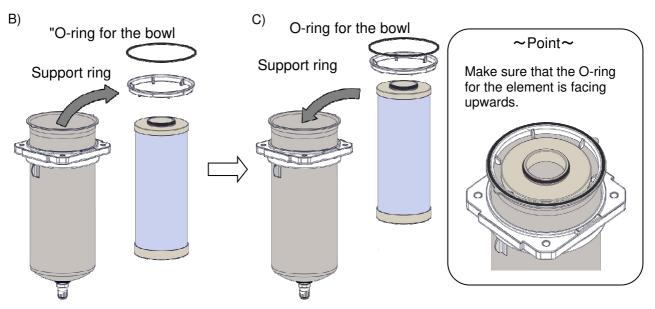
[When it is difficult to insert the new element into the body.]
