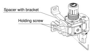
Tighten the 2 holding screws on the spacer with bracket or spacer evently. Tighten them to the recommended tightening torque. Insufficient tightening torque may result in loosening or sealing failure. Excessive tightening torque may damage the thread, etc.
