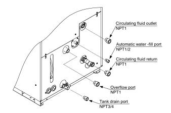
7) Operate the Thermo chiller and check that there is no fluid leakage after the sealant hardening.
