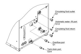
Operate the Thermo chiller and check that there is no fluid leakage after the sealant hardening.
