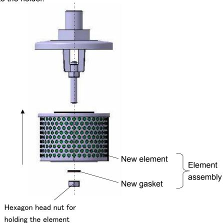
Screw in the element holding hexagon head nut.
