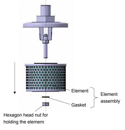
4. Replace the element and gasket with a new one, and mount them into the holder.
