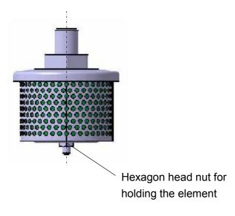
3. After removing the hexagon head screw, pull the gasket and element downward to remove them.
