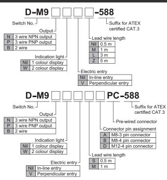
This product is a Solid State Auto Switch of direct mounting specification. Switch should only be used in areas in which potentially explosive atmospheres are unlikely to be present or only present for short periods of time
