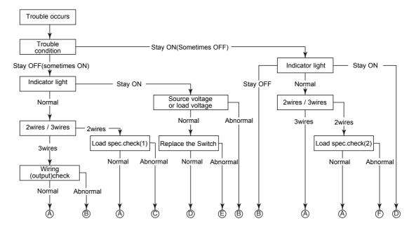
Load spec. check(1) ----- ON voltage > Load voltage-Internal voltage drop Load spec. check(2) ----- OFF current > Leak current
