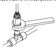
For one touch fittings, insert the tube into the sensor fitting carefully and securely all the way to the bottom.
