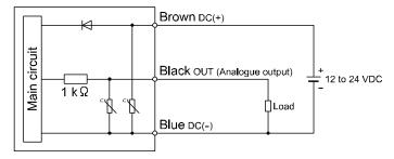
Analogue output: 1 to 5 V Output impedance: approx. 1  $k\Omega$
