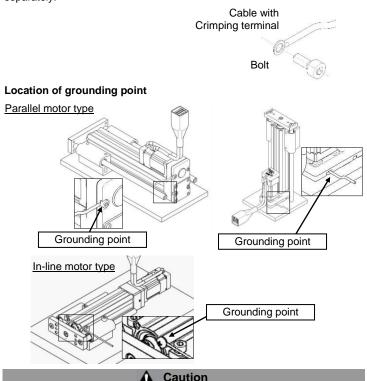
The product should be connected to a ground. The cross-sectional area of this wire shall be a minimum of  $2 \text{ mm}^2$ . The grounding point should be as near as possible to the actuator to keep the wire length short.
