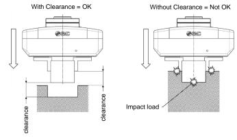
• When mounting a work piece, align it with the product carefully to prevent excessive force to the finger.
