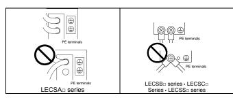
If an earth leakage circuit breaker is used, always connect the protective earth (PE) terminal of the driver to earth, to prevent an electric shock.
