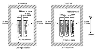
Note) Leave a large clearance between the top of the driver and the internal surface of a control box, and install a cooling fan to prevent the internal temperature of the control box from exceeding the environmental conditions.
