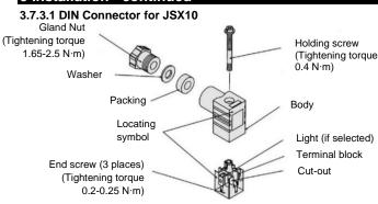
Figure 7. JSX10 DIN connector construction
