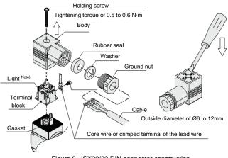
Figure 8. JSX20/30 DIN connector construction Note) The position is fixed regardless of the electrical entry direction.
