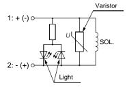
Figure 13. DIN terminal with light and surge voltage suppressor
