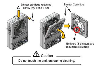
3) 8 emitters are mounted on the inside of the emitter cartridge. Clean
