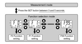
\*: Some products do not have all of the functions. If a function is not available or selected due to configuration of other functions, [- - -] is displayed on the sub display.
