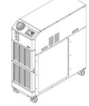
This product used a built-in pump to circulate a liquid such as water, adjusted to a constant temperature by the refrigeration circuit. This circulating liquid cools parts of customer's machine that generate heat.
