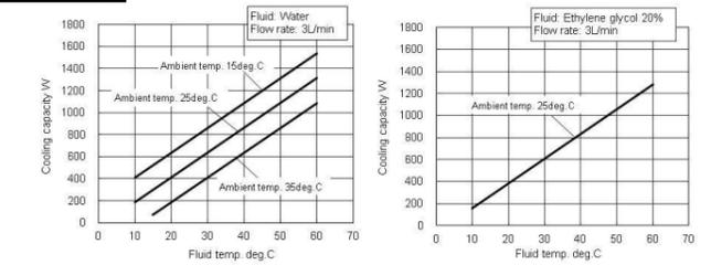
\*Cooling capacity decrease about 50W when high head pump option selected.
