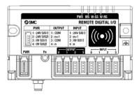
The intended use of this product is to provide a connection from the SMC wireless communication system to pneumatic devices.
