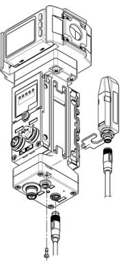
Mount the adaptor to the bracket of the Air Management Hub using the M10 nut already installed to the wireless adaptor (Recommended torque: 0.9 ±10% N•m).
