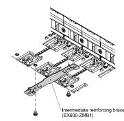
(2) Mount and tighten the end plate at one end of the unit and mount the intermediate reinforcing brace if required using M4 screws (Tightening torque: 0.7 to 0.8 N•m).
