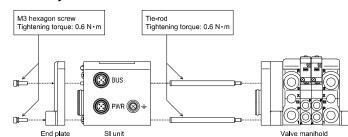
Hold the SI unit and the Input / Output blocks together in order to ensure there is no gap between them, while tightening the screws. Tighten the screws with the specified tightening torque (0.6 N•m).
