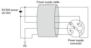
• SW power is supplied to the sensor connected to the input block. There is a voltage drop of approximately 1 V max. inside the SI unit when SW power is supplied. Select a sensor taking this voltage drop into consideration. If 24 V must be supplied to the sensor, it is necessary to increase the SW power supply voltage so that the input voltage of the sensor will be 24 V with the actual load (allowable SW power supply range: 19.2 V to 28.8 V).
