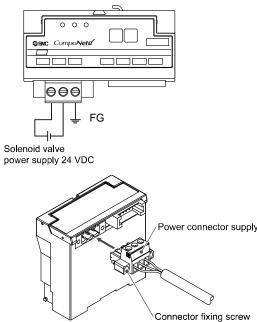
• Tighten the connector fixing screws (M2.5 screws) firmly with a tightening torque of 0.2 to 0.3 Nom.
